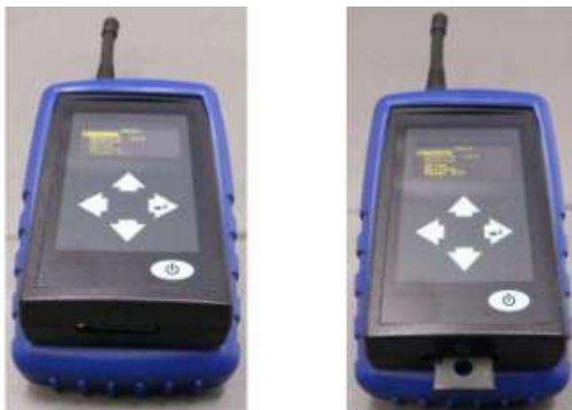
When no SIM card is fitted, the unit will display results for all networks detected.
