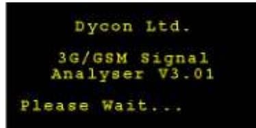
If any errors are detected during power-up, a GSM fault number will be shown (see section 18.1).
