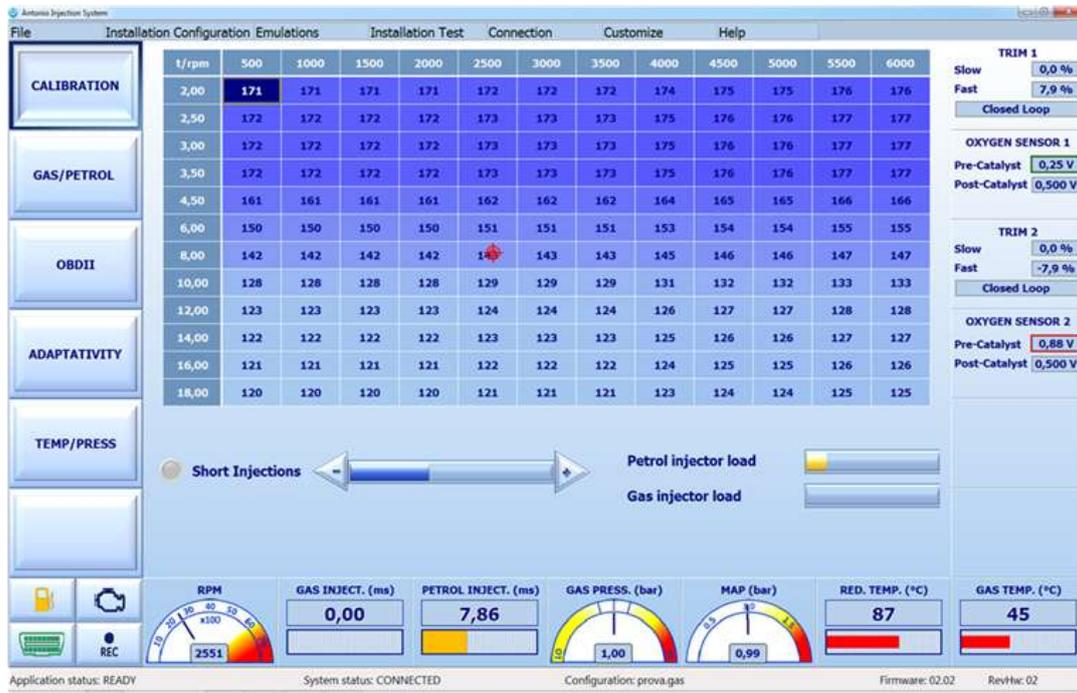
The calibration is made by setting a table of values, named as “**Gas Coefficients**”, which can be modified to make the right calibration of the vehicle avoiding that the petrol ECU notices a different working mode when running on gas.
