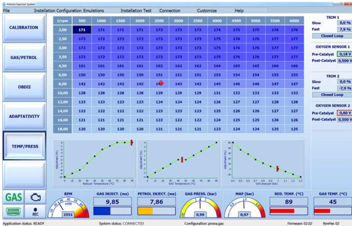
To apply these compensations you have to double click the blue spots on the displayed diagrams and enter the values of temperature or pressure and the related compensating percentage in the relative fields as shown in the following picture:
