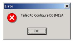
Ensure that the instrument is connected to the PC and that the correct drivers are installed, then re-launch the EasyLogger application.
