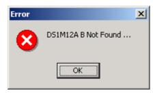
To resolve this, connect a DS1M12 to the PC and run the application again. If this has no effect, check that the drivers are installed correctly.
