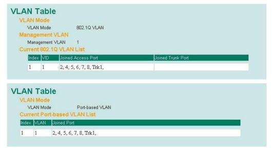
In 802.1Q VLAN table, you can review the VLAN groups that were created, Joined Access Ports, and Trunk Ports, and in Port-based VLAN table, you can review the VLAN group and Joined port.
