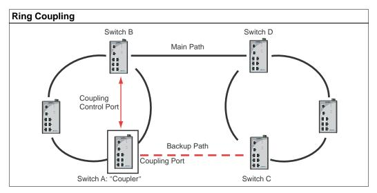
To support the Ring Coupling function, select two NI MES-3980 (e.g., Switch A and B in the above figure) in the Turbo Ring and another two NI MES-3980 in the adjacent Turbo Ring (e.g., Switch C and D).
