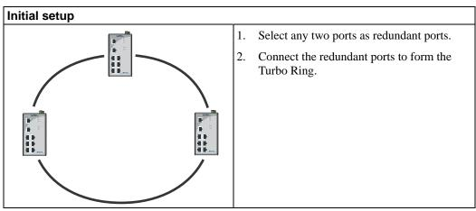
You do not need to set the Master to use Turbo Ring. Master is only needed to identify which segment acts as the backup path. The actual topology of the redundant ring, i.e., which segment will be blocked, is determined by the number of NI MES-3980 switches that make up the ring, and where the "Ring Master" is located.
