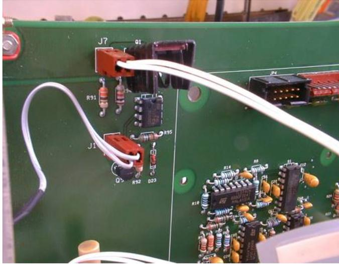
Figure 7. Disconnecting the lamp
