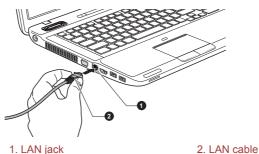
Figure 3-8 Connecting the LAN cable
