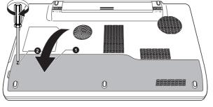
Figure 3-13 Seating the HDD/Memory module cover
