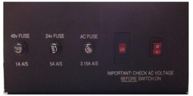
The sidecar uses an external linear dc power supply and the correct input voltage must be selected *before* connecting the power supply to ac power.
