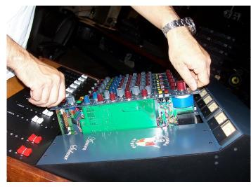
To remove the module, undo the two captive thrumb-screws and use them to pull the channel module from its connector and out of the Sidecar frame.
