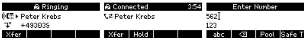
2. Enter the extension or other number on the keypad and press **✓**. While the phone is calling the number, you will either see the the hold screen (if you are transferring an active call) or a new missed call (if you are transferring a ringing call).
