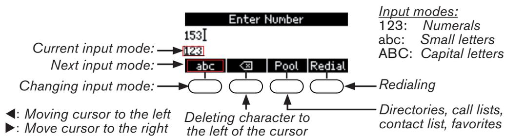
The current input mode is indicated in the information line. Press the left function key underneath the display to switch to the input mode indicated by the symbol directly above it in the function key line.
