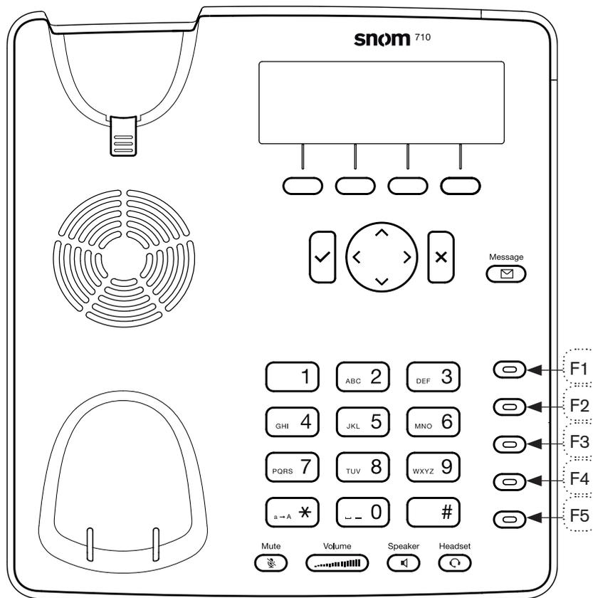
In the UC Edition firmware, the default setting of all programmable function keys with LEDs is line. See "Settings menu" on page 36 for the list of functions that can be selected for each key. The above diagram shows the location of the keys on the phone; the numbers F1 to F5 correspond to the list of keys in the phone's **Preferences** menu, submenu **Fkeys**, fkeys 1 - 5.
