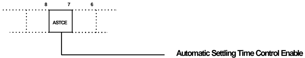
Figure 6 CONTREG Automatic Settling Time Control
