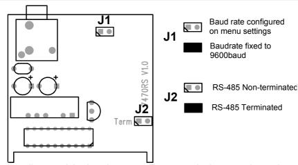
Jumper J1 should be normally open. It is closed when the 7470 baud rate is not known, to force 9600 baud.
