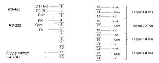
The green connector blocks are detachable to make connecting easier. They accept up to 2.5mm<sup>2</sup> wires.
