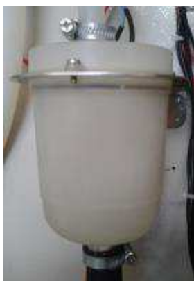
Floating water level detection device
