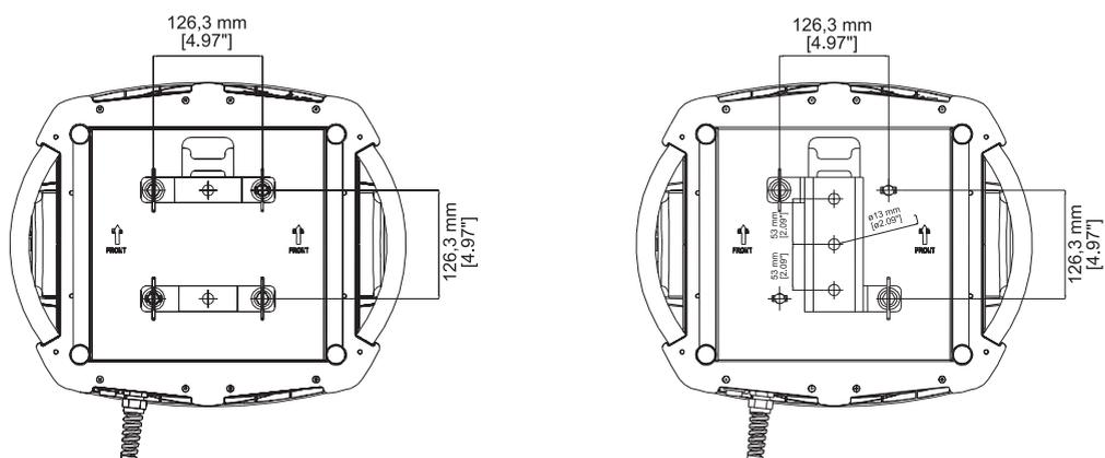
For ceiling mounted installations we suggest the use of appropriate clamps or fixings to attach the fixture to the mounting surface. Clamps may be attached to the central hole provided in the cam-lock brackets, as shown in the following diagram.
