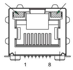
To Maximise the EMI performance the unused (N/C) conductors will be terminated with  $75\Omega$  and 1.5nF to the RJ45 shield.
