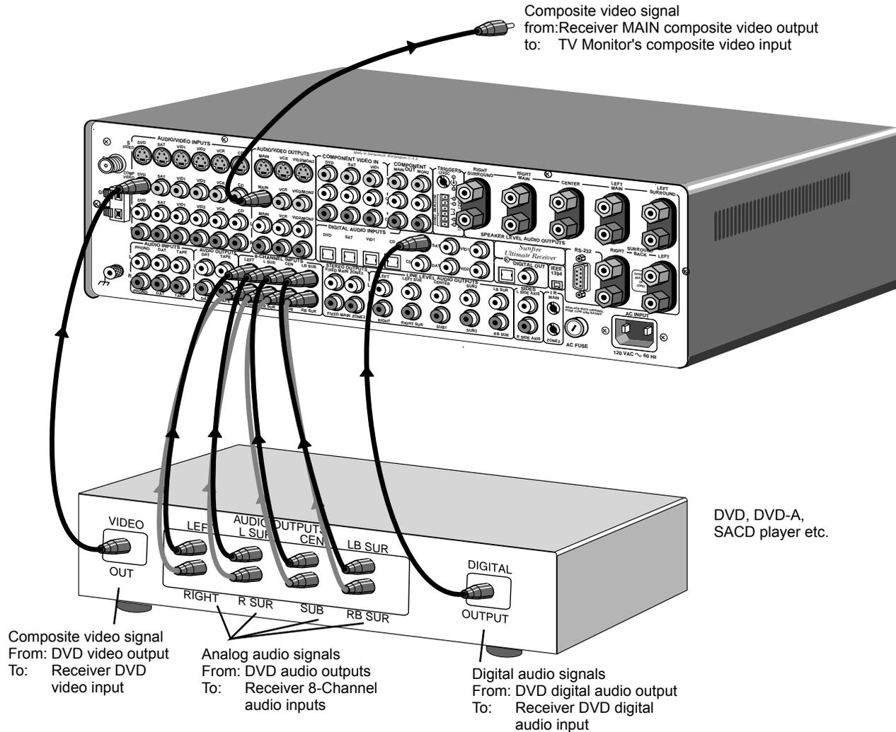
This input is really useful as an input for DVD A, SACD, etc., as a multichannel direct (DSP-bypass) input.
