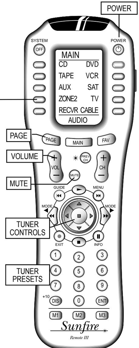
Note: Zone 2 can also be turned on and adjusted without using the remote. Press the Zone 2 button on the Receiver's front panel, followed by Power, to turn it on (or off), or adjust the input source or volume.
