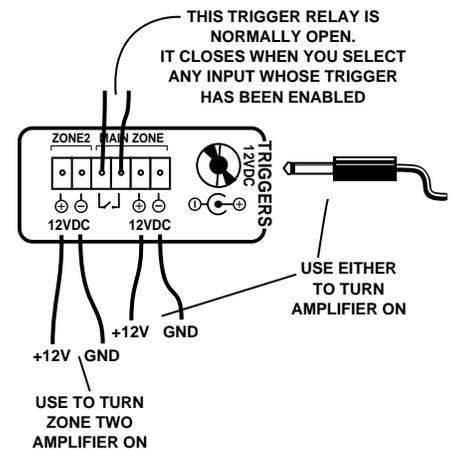
DO NOT use the relay contacts for 120 VAC or 240 VAC switching! They are only for low voltage AC/DC loads of 2 A maximum.
