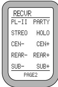
4. The following buttons with fixed labels are also programmed: Power, Volume up, down and Mute. The number pad accesses the tuner presets directly, and CH+/- steps through them. DIS is the +10 function, and ENT is station enter. The MODE buttons either side of the joystick, allow you to select the different surround modes.
