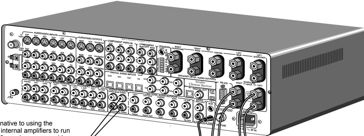
As an alternative to using the Receiver's internal amplifiers to run your Zone 2 speakers, you could use an external power amplifier. Connect the amplifier's line-level inputs to the Receiver's Zone 2 stereo outputs.
