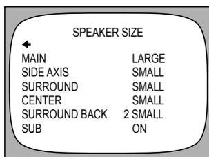
Use the joystick pad to set the size of each speaker to Small or Large, or set to Off for those speakers which are not present. Return to the SPEAKERS Menu when you are finished.
