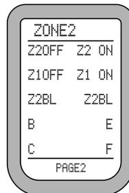
**Note:** Zone 2 must first be enabled using the OSD (see page 36), or these controls will have no effect. Zone 2 can be turned on even if the Main Zone is off.
