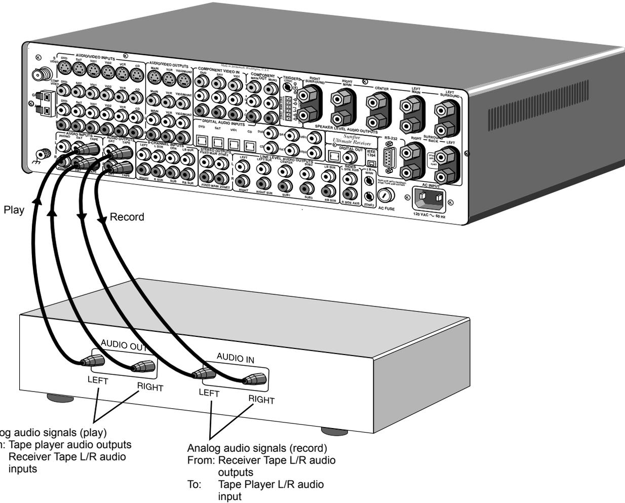
The Tape player's output can be connected to the TAPE or DAT inputs. If you have two players, the Receiver will automatically select the input which has a signal present. The unused deck must be turned off when the other deck is playing.
