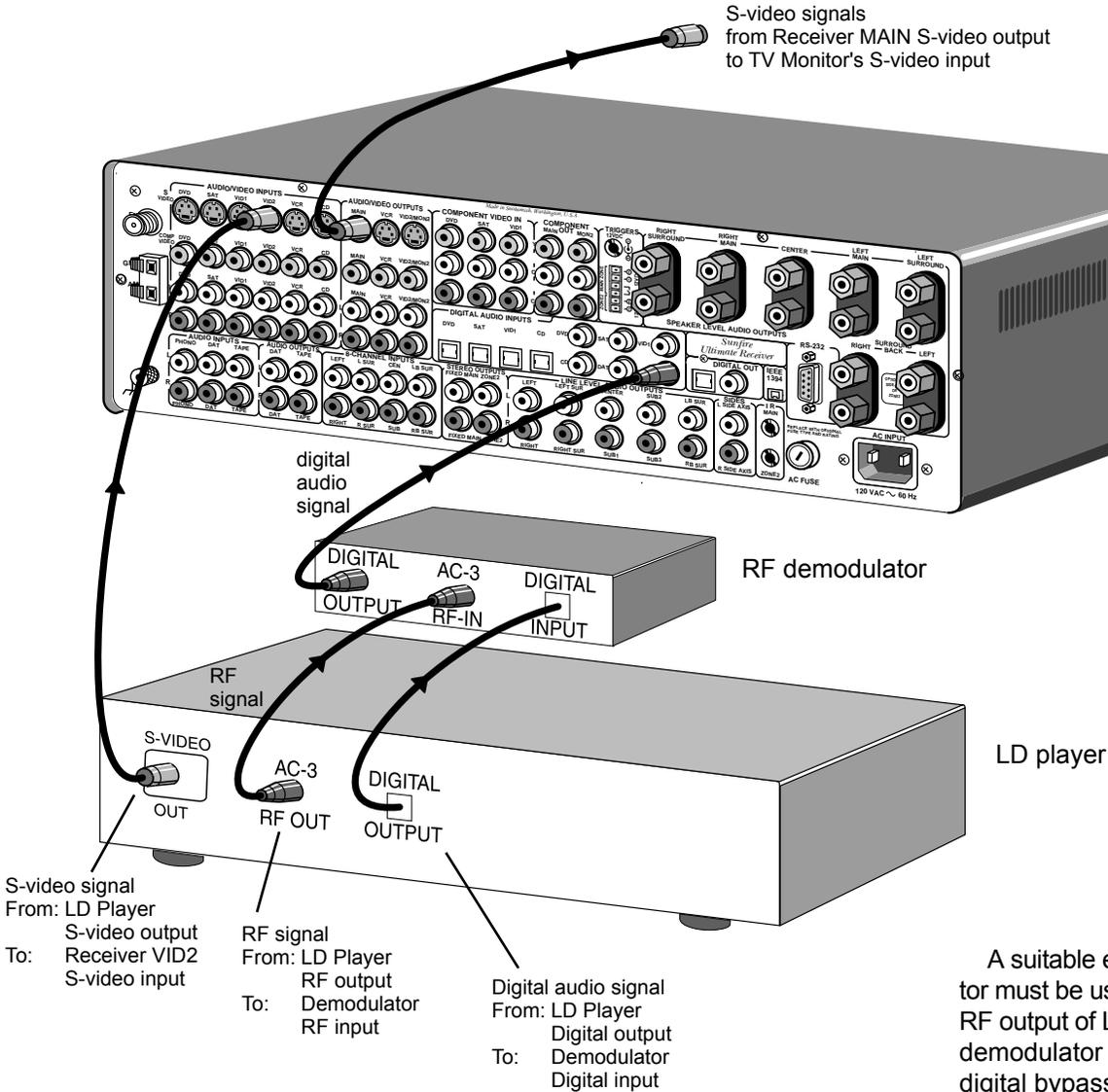
A suitable external RF demodulator must be used to convert the AC-3 RF output of LD players. Ideally, the demodulator should also have a digital bypass (pass-through) feature. Lexicon and B&K are among several companies making excellent demodulators with this feature.
