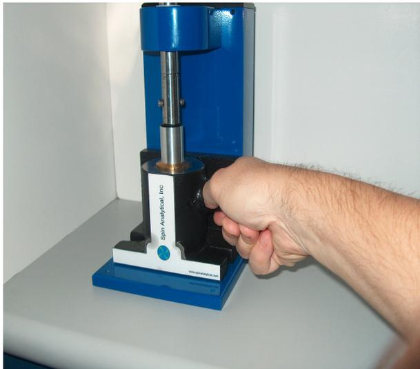
**Figure 4: Closing collet with shaft engaged**
