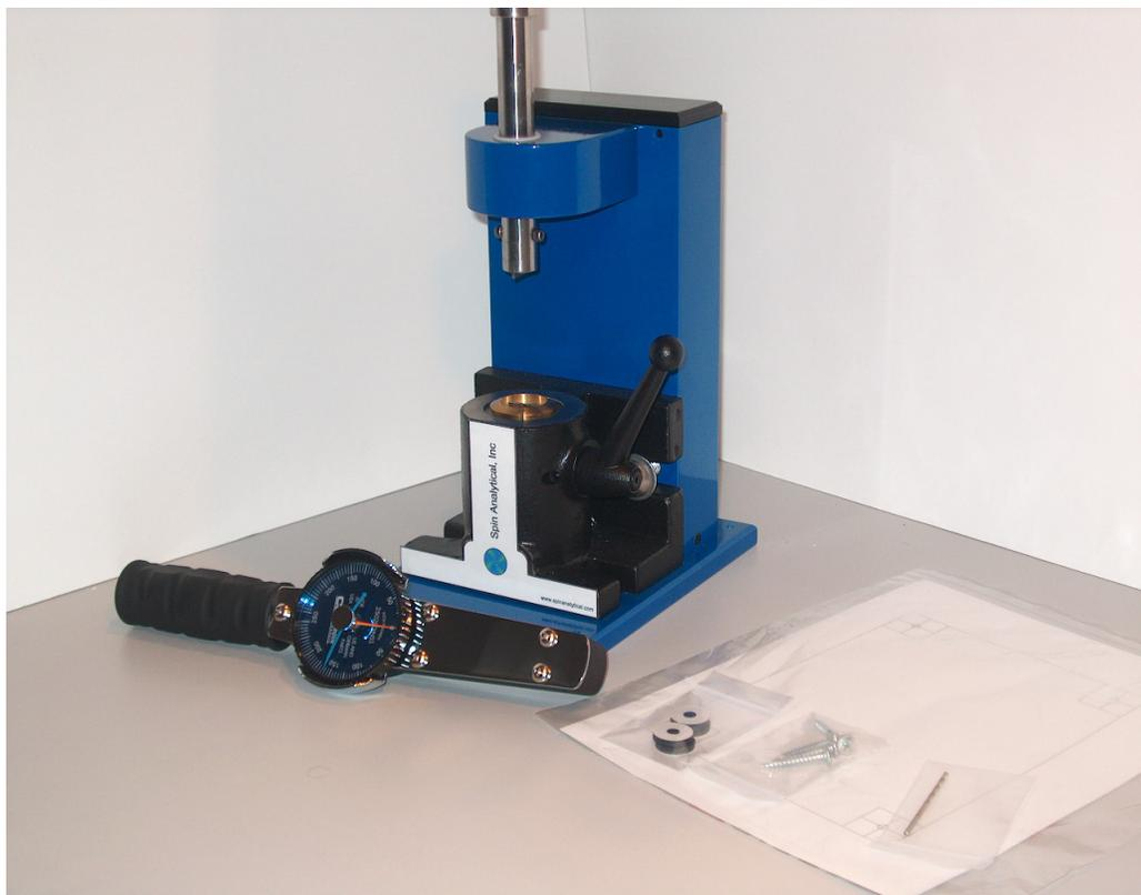
Figure 1: Components included with AUC Cell Assembly Torque Stand
