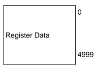
Data contained in this database is paged through the input and output images by coordination of the ControlLogix ladder logic and the MVI56E-MNETR module's program. Up to 40 words of data can be transferred from the module to the processor at a time. Up to 40 words of data can be transferred from the processor to the module. Each image has a defined structure depending on the data content and the function of the data transfer. The module uses the following block numbers:
