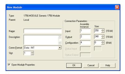
Enter the Name, Description and Slot options for your application. You must select the **COMM FORMAT AS DATA - INT** in the dialog box, otherwise the module will not communicate over the backplane of the ControlLogix rack. Click OK to continue.
