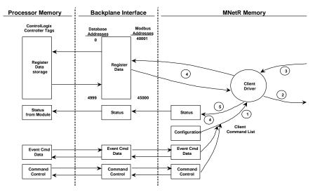
1 The client driver obtains configuration data from the MNET.CFG file when the module restarts. The configuration data obtained includes the timeout parameters and the Command List. These values are used by the driver to determine the type of commands to be issued to the other nodes on the Modbus TCP/IP network.
