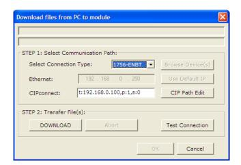
2 Configure the path as shown in the following illustration, and click CONSTRUCT CIP PATH to build the path in text format.
