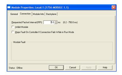
3 Save the module. Click OK to dismiss the dialog box. The CONTROLLER ORGANIZATION window now displays the module's presence.
