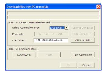
2 Configure the path as shown in the following illustration for this example and click **CONSTRUCT CIP PATH** to build the path in text format.
