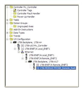
Note. If you are installing the MVI56E-MNETR module in a local rack, follow these steps. If you are installing the module in a remote rack, refer to Create the Module - Remote Rack (page 27).
