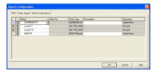
**10** Associate the I/O connection variables to the correct module. The default values are Local:1:I and Local:1:O so these require change.
