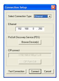
3 If PCB is still unable to connect to the module, click the BROWSE DEVICE(s) button to open the PROSOFT DISCOVERY SERVICE.
