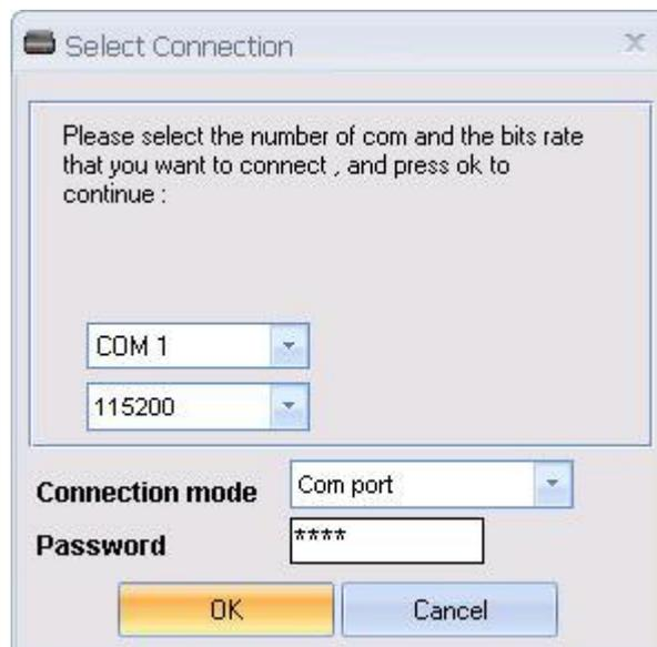
4) Select the Com Port to which the Router is connected to, the connection frequency should be **115200**, the **Connection mode** should be via **Com port** and the default **Password** is **0000**.
