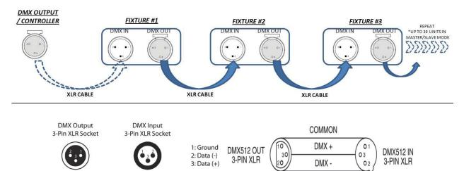
For installations where the DMX cable has to run a long distance, or is in an electrically noisy environment, it is recommended to use a DMX terminator. This helps in preventing corruption of the digital control signal by electrical noise. The DMX terminator is simply an XLR plug with a 120  $\Omega$  resistor connected between pins 2 and 3,which is then plugged into the output XLR socket of the last fixture in the chain. Please see illustrations below.
