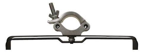
Regardless of the rigging option you choose for your MICROH UV BRICK16 wash fixture, always be sure to secure your fixture with a safety cable. The fixture provides a built-in rigging point for a safety cable on the hanging bracket as illustrated above. Be sure to only use the designated rigging point for the safety cable and never secure a safety cable to a carrying handle.
