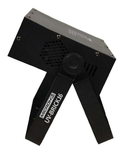
**Clamp Mounting:** The MICROH UV BRICK16 provides a unique mounting bracket assembly that integrates 2 brackets to be used to mount on a truss or the floor. When mounting this fixture to truss, be sure to secure an appropriately rated clamp to the included bracket fitted through the center hole. As an added safety measure, be sure to attach at least one properly rated safety cable to the fixture.
