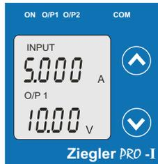
Screen 4 : Current Input and Output 1 as Current
