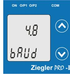
This screen allows the user to set Baud Rate of RS 485 port. The values displayed on screen are in kbaud ..
