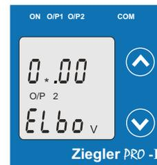
Enter New / Change Elbow value of the Output 2, first digit entered, prompting for second digit. (\*Denotes that digit will be flashing).
