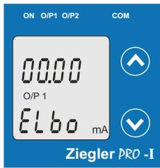
Pressing the "Down" key will enter the "New/Change Elbow value of the Output 1edit" mode.
