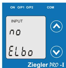
Pressing the "Down" key will enter the "Selection of Elbow function of Input edit" mode and scroll the value between yes and no.
