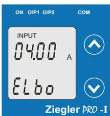
Pressing the "Down" key will enter the "New/Change Elbow value of the Input edit" mode.
