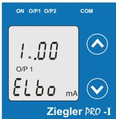
Enter New / Change Elbow value of the Output 1, first digit entered, prompting for second digit. (\*Denotes that digit will be flashing).
