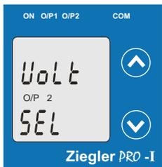
Pressing the "▼ Down" key will enter the "output 2 type edit" mode and scroll between voltage and current.
