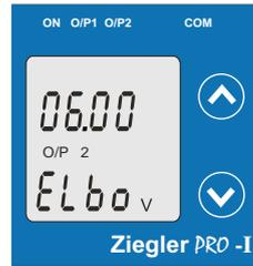
Pressing the "Down" key will enter the "New/Change Elbow value of the Output 2 edit" mode.
