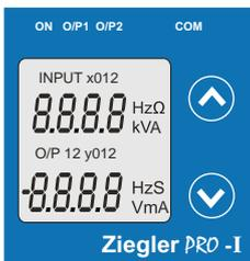
Ziegler PRO - I can be configured and programmed at site for the following : CT Primary ,CT Secondary (5A or1A) , Input parameters (i.e start, end and elbow value of Input) and Output parameters(i.e as Voltage or as Current and start, end and elbow value of outputs).
