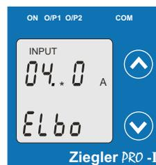
Enter New / Change Elbow value of the Input, second digit entered, prompting for third digit. (\*Denotes that digit will be flashing).
