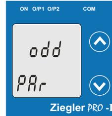
Pressing the "Down" key will enter the "Parity & stop bit edit" mode and scroll the value through
