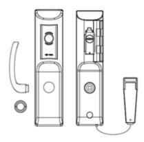
Remove the front cover and lever first. Insert the J2.5 plug of the record reader into the hole of lock under outside cover and turn on the power of record reader, red indicator light is. Then place any card in the reading area of the lock, the red indicator light of record reader and LED light on lock keep flashing for 30 seconds and it starts to read data. After "di-" sound, it means reading over. Please turn off the power of record reader and unplug it from the lock.
