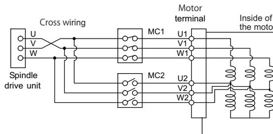
MC1: Contactor to connect low-speed coil (1st  $\blacktriangle$ -connection)
