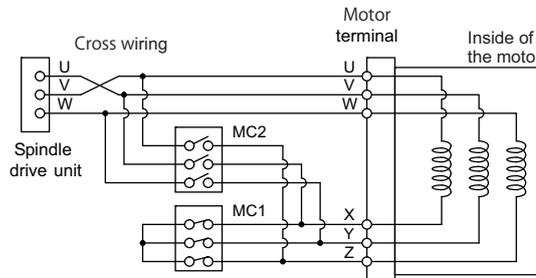
MC1: Contactor to connect low-speed coil ( $\blacktriangle$ -connection)
