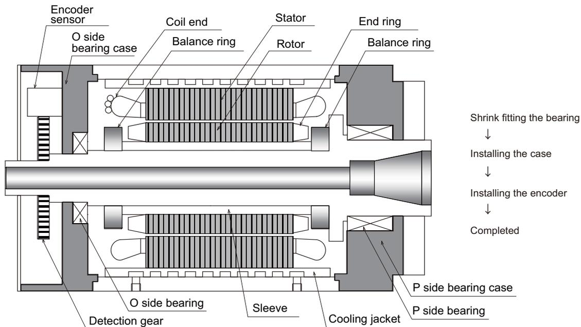
**(1) Ensuring the space for the stator coil end**
