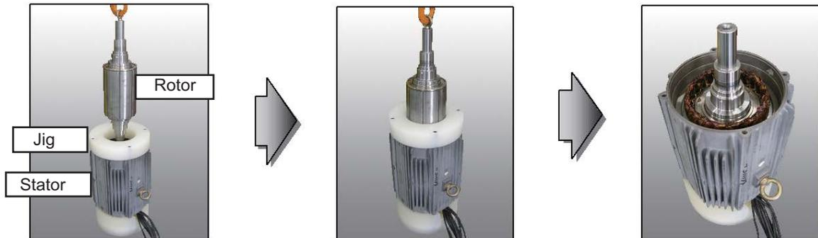
Example of assembling a rotor
