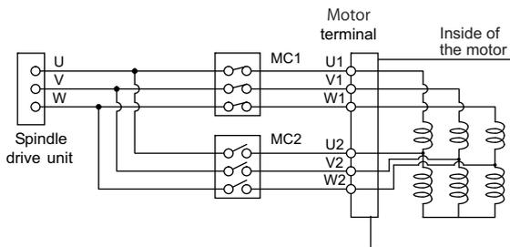
MC1: Contactor to connect low-speed coil (1st  $\blacktriangle$ -connection)
