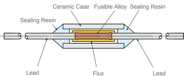
The leads of the SM-type are connected by a fusible alloy thereby allowing the current to flow directly from one lead to the other. The fusible alloy is coated with a special flux.
