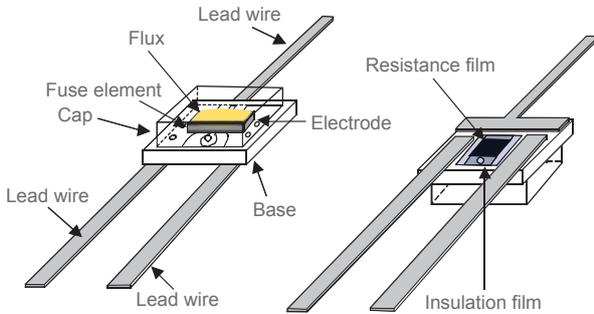
The D6-type houses a printed electrode, a fuse element and a special flux material in layers on top of the ceramic base. The current flows from one lead, across the fuse element and then through the second lead.
