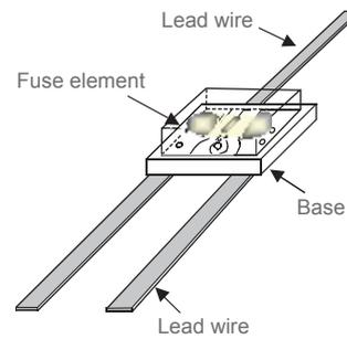
When the ambient temperature rises to the operating temperature of the D6-type, the fuse element melts, and forms a drop around the end of each lead because of surface tension and the special flux coating. This cuts off the electrical circuit. In another scenario, the heater resistance generates heat in response to an external signal, thereby melting the fuse element and cutting off the electrical circuit immediately.
