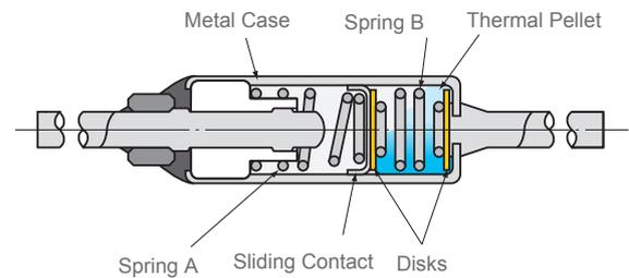
When the ambient temperature rises to the operating temperature of the SF-type, heat is transferred through the metal case and melts the thermal pellet. Springs A and B then stretch and the sliding contact moves away from lead A, thereby opening the electrical circuit.
