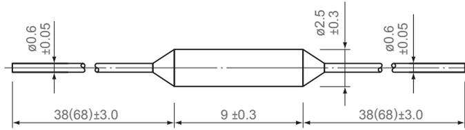
Note: The dimensions for long lead devices are in parentheses.
