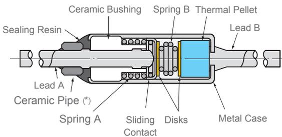
The SF-type contains a sliding contact, springs and a thermal pellet inside a metal case. When spring B is compressed, there is firm contact between lead A and the sliding contact. At normal temperatures, current flows from lead A to the sliding contact and then through the metal case to lead B.
