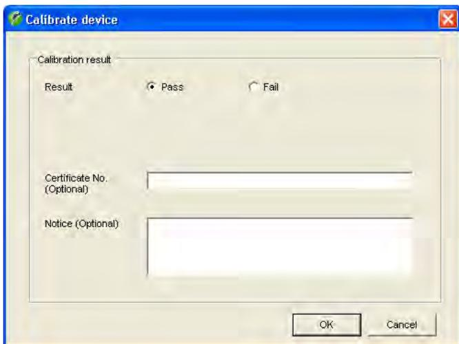
If you wish to enter the **adjustment data** of a barometer, hygrometer or thermometer, select the respective device from the list and then click on the **"Calibrate"** button. The window shown at left appears and you may enter the result of the adjustment ("Pass" or "Fail"). In addition, you may enter the number of the certificate as well as a notice.
