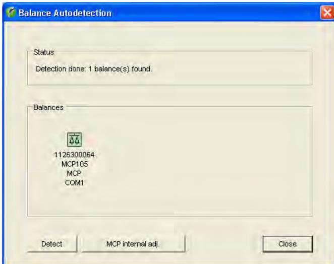
Every time the application is launched, Calibry automatically checks the balances that are connected to the PC and ready for operation, and displays the results in the status area. Balances that are readily available to Calibry are shown in the lower part of the window. The balance check may be repeated as needed by clicking on "**Detect**". If the results of the check prove to be OK you may click on "**Close**" to start working with Calibry.
