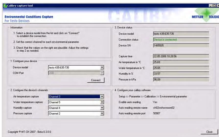
The Calibry Capture Tool will automatically recognize the connected measuring instrument and display the respective data in the “Device status” section of the window.
