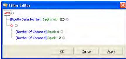
This menu also contains the option "Add Group", which you can use to define a subgroup for the filter. Opposite is an example for filtering with a subgroup. In this example, after filtering, only pipettes whose serial number begins with "123" or which have 8 or 12 channels are displayed in the list.
