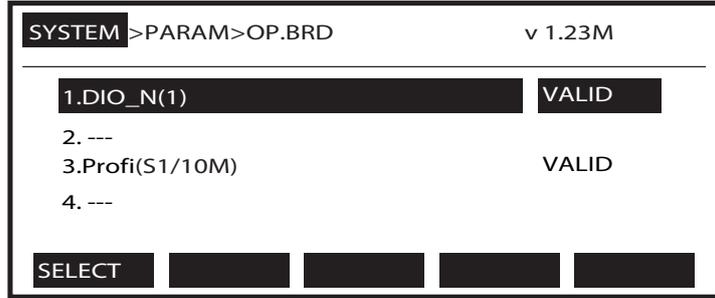
Option boards installed into the option slots are displayed on the PB screen.
