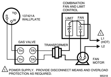
**Fig. 5—T87F replacing a Series 10 Thermostat connected to a 3-wire, open-contact, high-limit control.**
