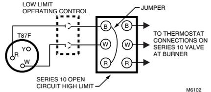
**Fig. 6—T87F used for Series 20, 3-wire, spdt control of low-voltage motors and electric radiator valves. Used in applications where thermostat makes contact on both a rise and fall in room temperature.**
