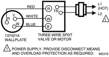
**Fig. 7—T87F used in cooling-only system.**
