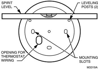
**Fig. 2—Mounting wallplate or subbase to wall.**
