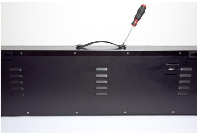
Figure 18 - Unscrew the two handle screws
