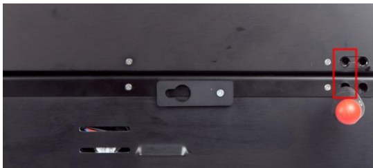
Figure 22 - Do not insert first one pin and then the other one
