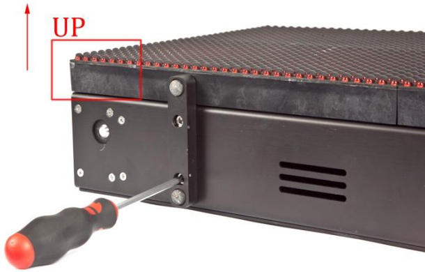
Figure 20 - Unscrew the two foot screws
