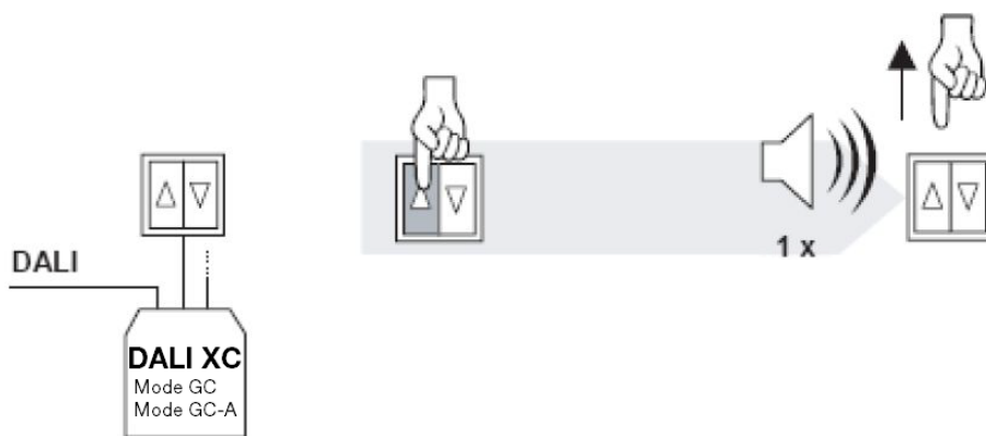
Figure 9: Assigning a luminaire to a group
