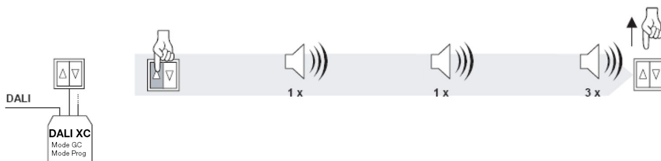
Figure 12: Finishing system extension
