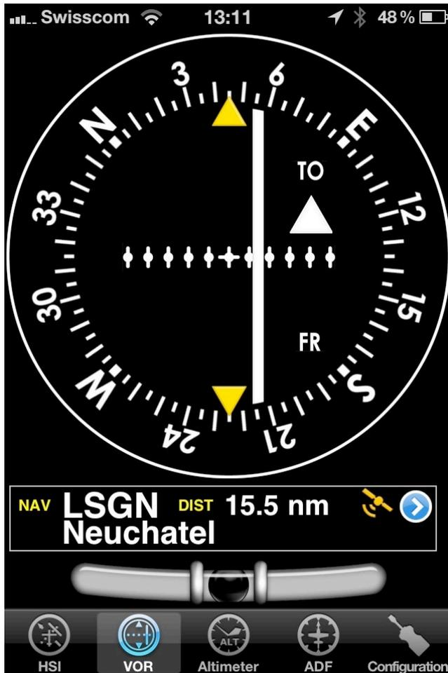
The VOR instrument uses GPS data to display the bearing to a waypoint
