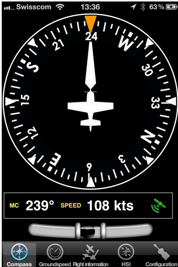
The “compass” instrument displays the current GPS course (not the magnetic heading) on a virtual animated compass card. The course can be displayed either as true course or magnetic course depending on the settings.
