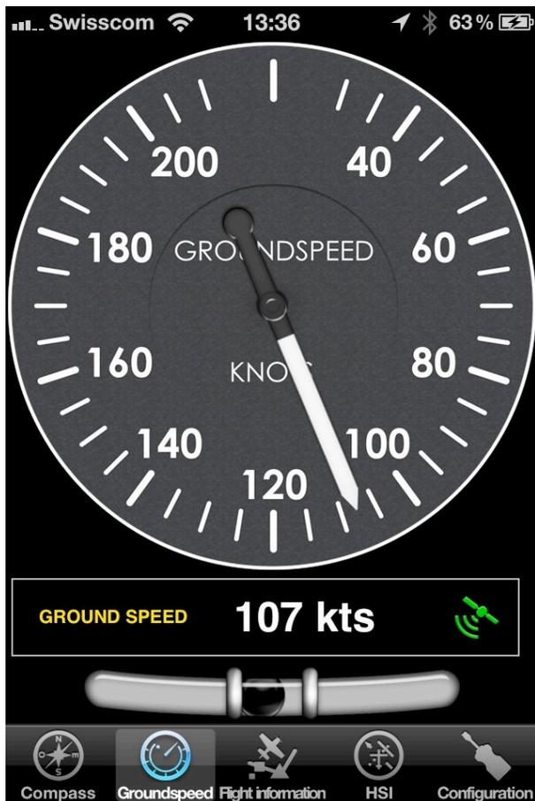
The top part is the analog ground speed indicator. On the bottom part you will find the digital speed value as well as the current GPS status symbol.
