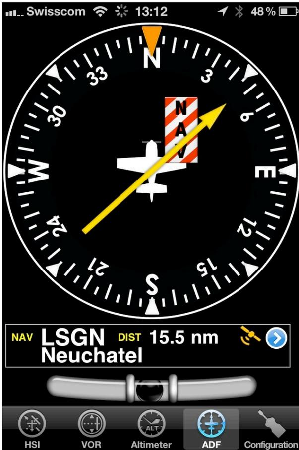
The ADF instrument in Air Navigation uses GPS track information and does of course not receive any radio waves. It can still be of value for practicing ADF navigation.
