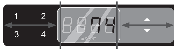
Figure 4: Activating and deactivating the keylock can be done by swiping left or right underneath the display
