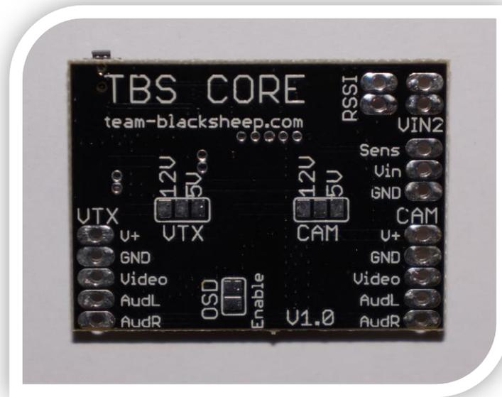
The output voltage is set by joining the center solder pad and the left (12V) or the right (5V) of the VTx and Camera ports respectively. If you are planning to use a third-party OSD, you can already proceed to the next step. To enable the OSD on your TBS CORE, connect the two pads at **OSD**. Instructions for configuring the TBS CORE OSD are provided in the next chapter.
