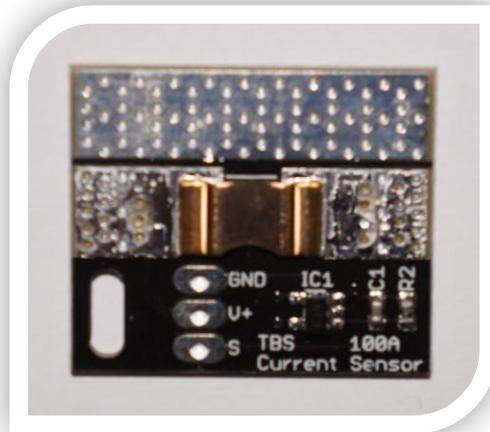
The current sensors come in two flavors, 50A and 100A. The 50A is more accurate at lower voltages. Wire the current sensor between your battery plug and ESC. Please be careful to install it in the right direction, copy below image carefully. When pulling a lot of power, spread some solder to fill up the holes.
