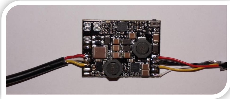
On the TBS CORE, pre-tin the solder pads with a bit of solder. Verify once again that the pinout is correct, position the wire above the pre-tinned pad and apply heat to the solder pad on the TBS CORE. Repeat for all cables that you want to connect, and you're done. To save space and make life easier, you can solder at both the front and the back.
