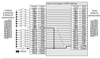
If your system is set to run on a rated input voltage of 12VDC when you make a switch from A1SX40 to QX40, it must be reset to run on 24VDC
