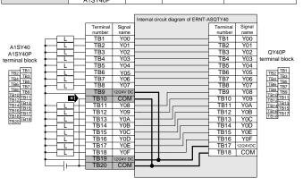
Because the switch concerned causes the number of points per common to change from 8 (two circuits) to 16, an alteration to the wiring is required if the terminal numbers TB9 and TB19, and TB10 and TB20, on the MELSEC-AnS-side terminal block have been used in separation from each other.
