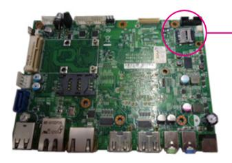
The default 8GB Micro SD card is installed in NDiS 102 with pre-configured Uboot and filesystem. User can also use their own Micro CD card to build different configuration files according to their development environment.
