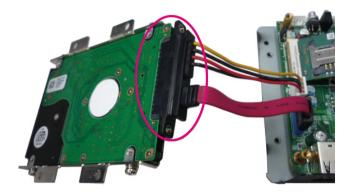
4. Use the provided screws to secure the SATA drive in place and secure the SATA Drive with the provided mounting screw.
