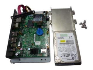
2. Place the SATA hard drive onto the drive bracket. Align the mounting holes that are on the sides of the SATA drive with the mounting holes on the drive bracket.
