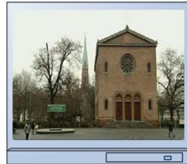
Anamorphically distorted 16:9 TV picture on 4:3 TV screen
