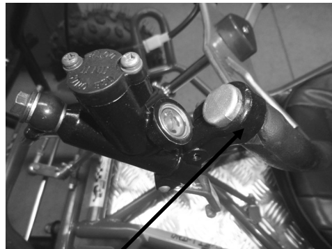
Fig.8 Hydraulic brake clamp attachment to steering wheel. Use allen key to tighten.
