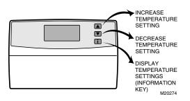
2. To raise the temperature setting, press the A key. When in the cooling mode, raising the temperature before you leave for work or school also lowers. your energy costs.
