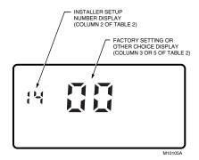
Fig. 12. Display of Installer Setup and setting.
