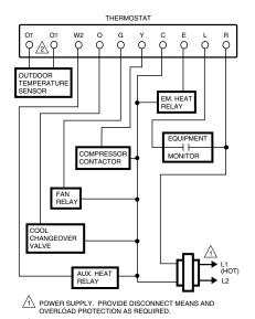
Fig. 4. Typical hookup in heat pump system with emergency heat relay.
