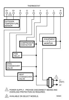
Fig. 3. Typical hookup in heat pump application.
