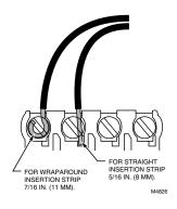
Fig. 6. Proper wiring technique.
