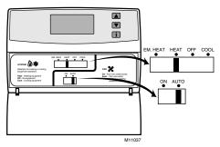
Fig. 9. T8511R (manual changeover) system and fan switches location.
