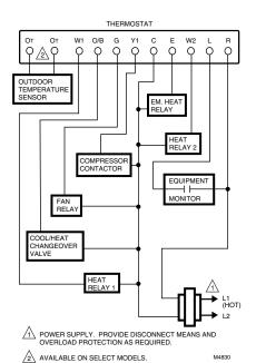
Fig. 5. Typical hookup in heat pump application with emergency heat relay and O/B terminal.
