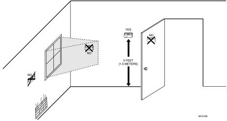
Fig. 1. Typical location of thermostat.
