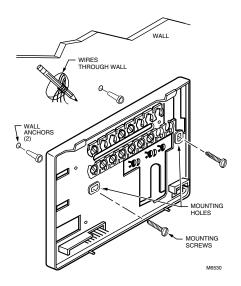
Fig. 2. Mounting the wallplate.
