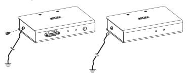
2. Make sure that the computer that the CE250AL connects to and the monitor that the CE250AR connects to are properly grounded.
