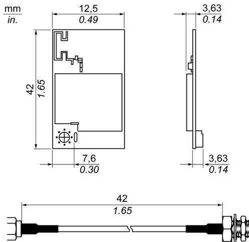
**NOTE:** The interface is mounted on a USB cable available within the product. The antennas are mounted directly on the product to locations in the bottom (see page 22). They can also be mounted remotely using intermediate cables.
