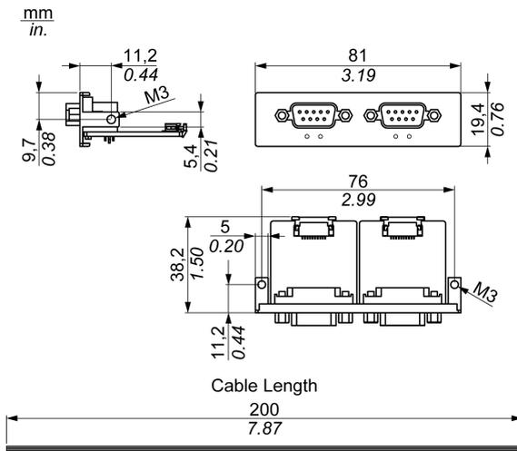
The following figure shows the dimensions of the 4 x RS-232/422/485 interface module:
