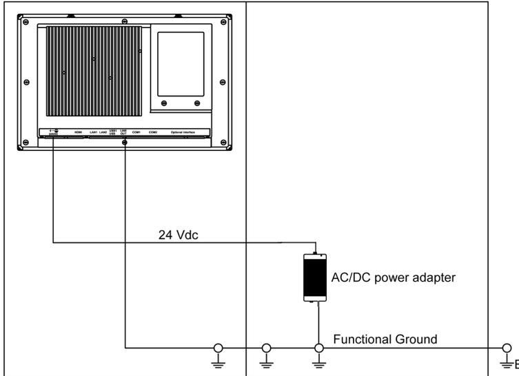
Use the AC/DC power adapter for connecting the Industrial Personal Computer.
