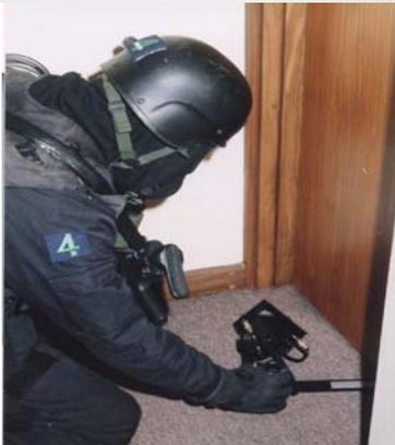
Cameras: Watec 902 1/3" CCD 570 lines 0.00009 lux (MK2) or Night Vision Star 300 1/3" with image integration CCD 580 lines 0.00005 lux (MK3)
