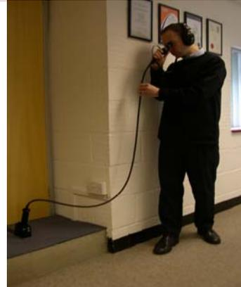
Fibreoptic Cable: High Resolution 30K Pixel, 1500mm long leading to focussing eyepiece which allows the operator to stand well away from the door
