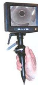
Snap locks to Videoscope head augments or can replace MP500 screen
