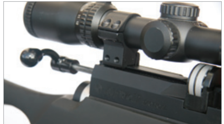
The bolt doesn't cock the rifle, rather allows the magazine to index around, then when pushed in probes a pellet into the breech
