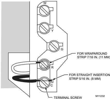
Fig. 4. Wiring connections.
