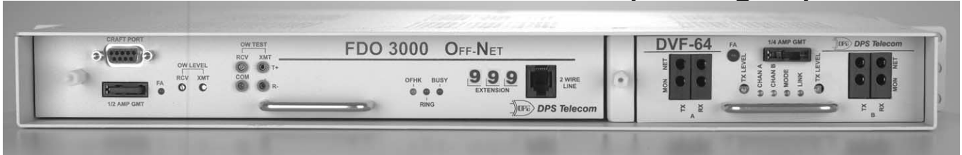
Fig. 1 - FDO 3000 Off-net with DVF-64 digital VF interface card provides telephone network interface for order-wire on 64 Kbit service channel.
