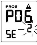
**< OK >** Confirm value of SERVICE parameter (2 = control for H/C, MOD2 in this case)
