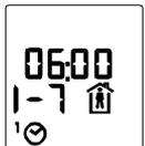
Display for a switching command in the weekly switching programme.
