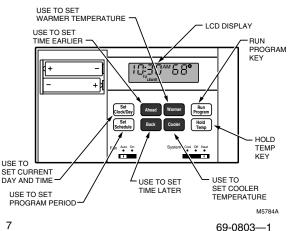
Use the **Time** keys to program WAKE time and use the **Temp** keys to program the WAKE temperature for Mon-Fri. Repeat the sequence for LEAVE, RETURN, and SLEEP.
