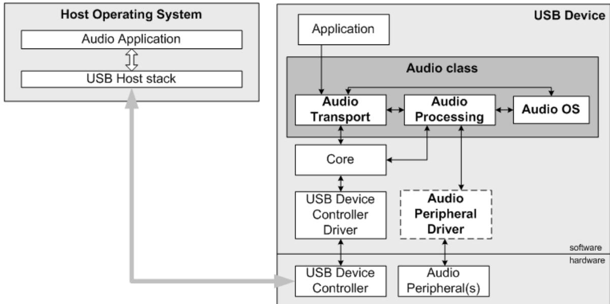
Figure - General Architecture between a Host and Micrium's Audio Class
