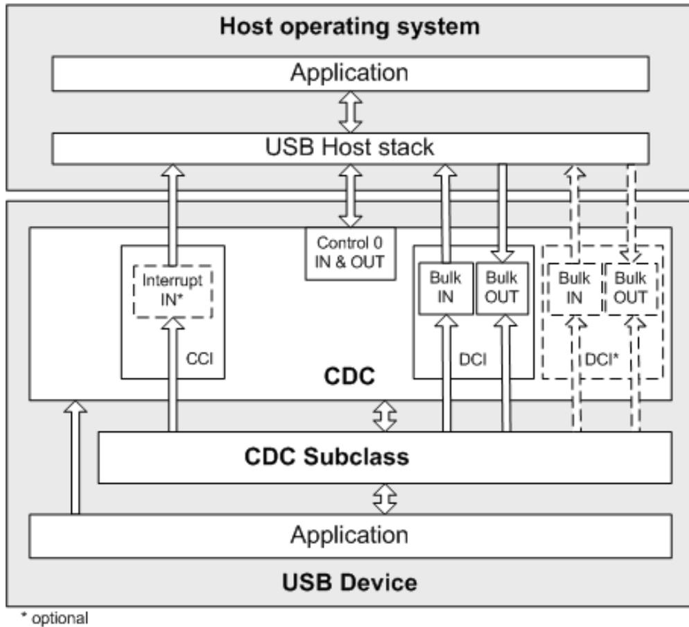
Figure - General Architecture between a Host and Micrium's CDC Class
