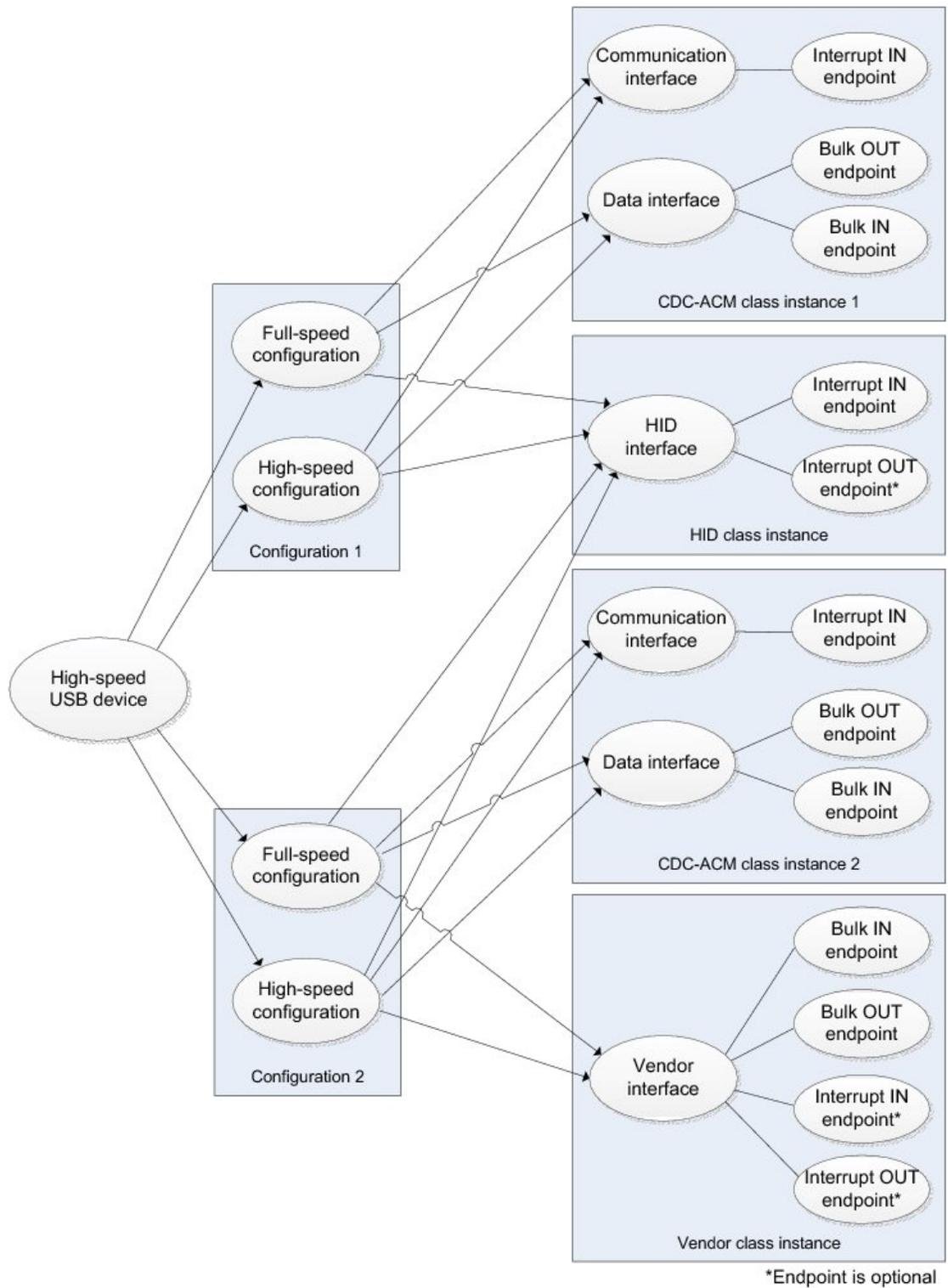
Figure - Complex Composite High-Speed USB Device Structure
