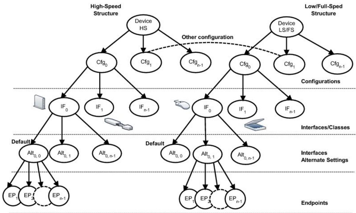
Figure - USB Device Structure
