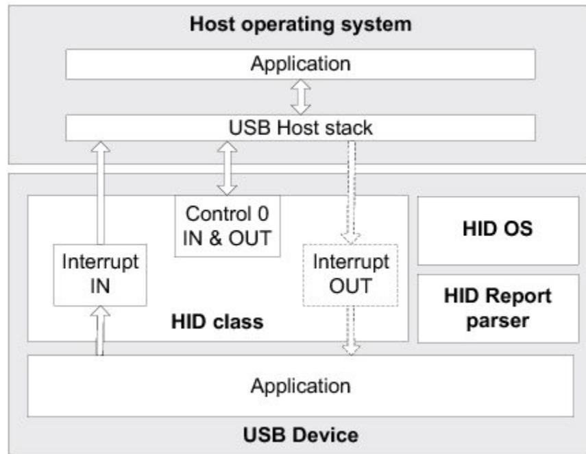
Figure - General Architecture Between a Host and HID Class
