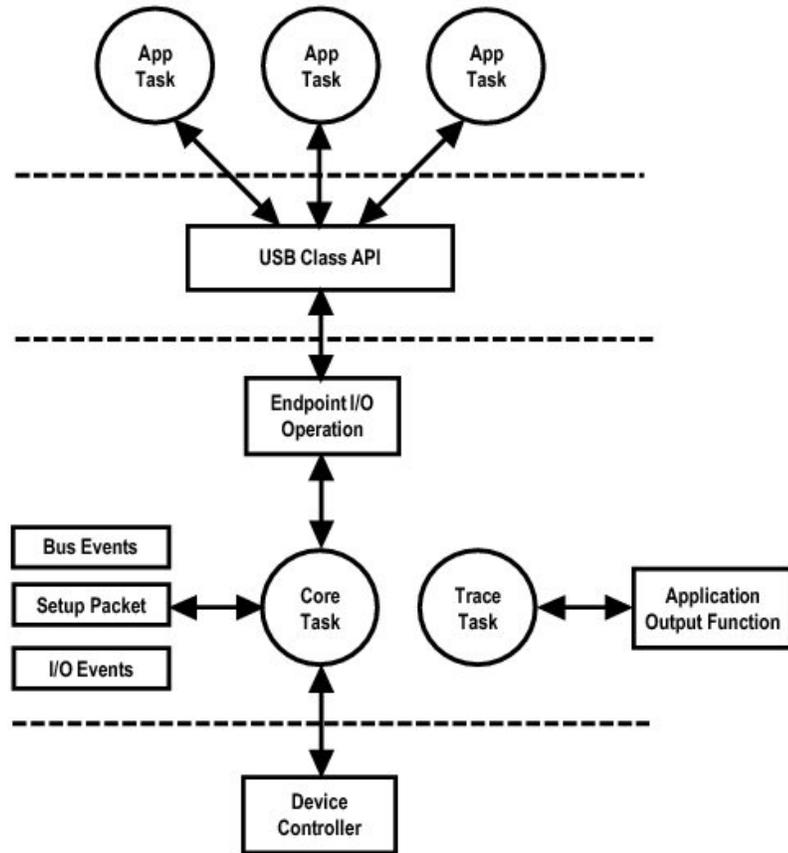
Figure - µC/USB-Device Task Model
