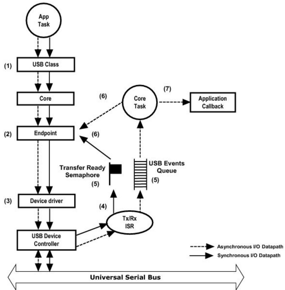
Figure - Sending and Receiving a Packet
