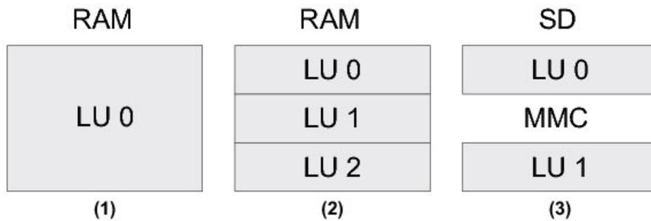
Figure - Example of Logical Units Configurations
