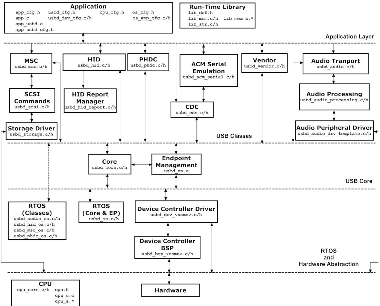
Figure - µC/USB-Device Architecture Block Diagram
