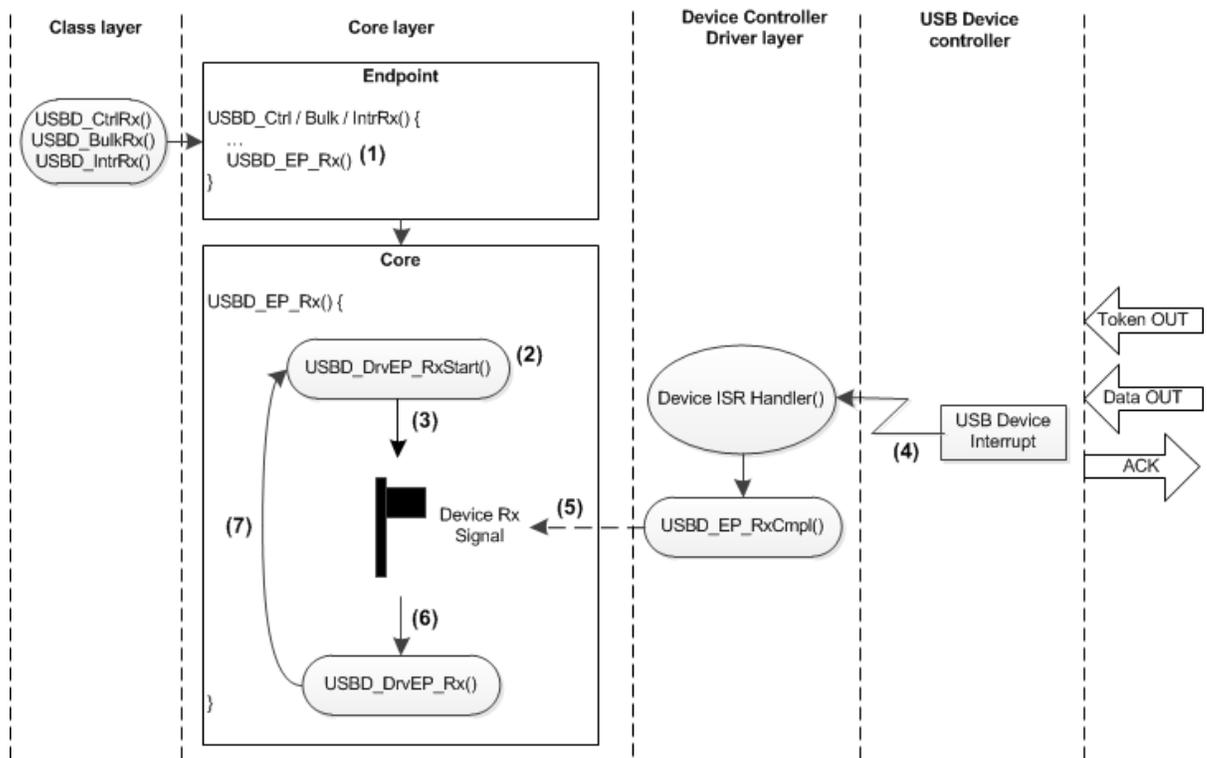
Figure - Device Synchronous Receive Diagram
