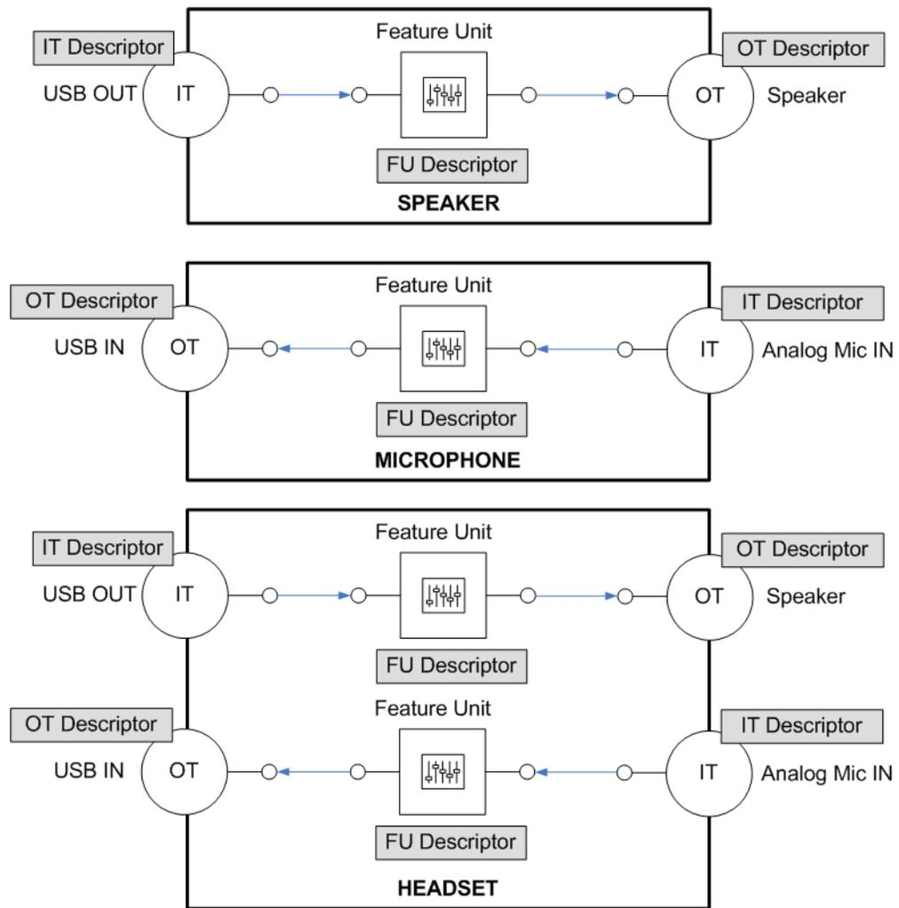
Figure - usbd\_audio\_dec\_cfg.c - Typical Topologies Example
