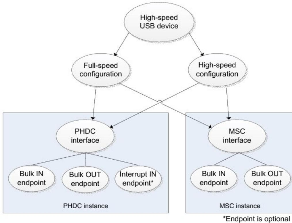
Figure - Composite High-Speed USB Device Structure
