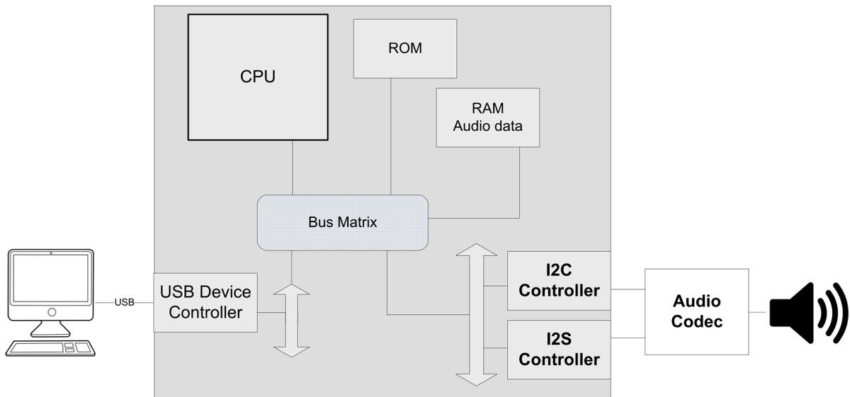
Figure - Typical Audio Codec Interfacing a MCU
