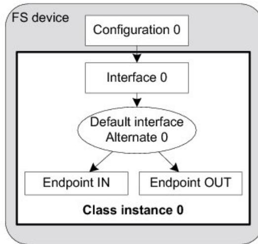
Figure - Multiple Class Instances - FS Device (1 Configuration with 1 Interface)
