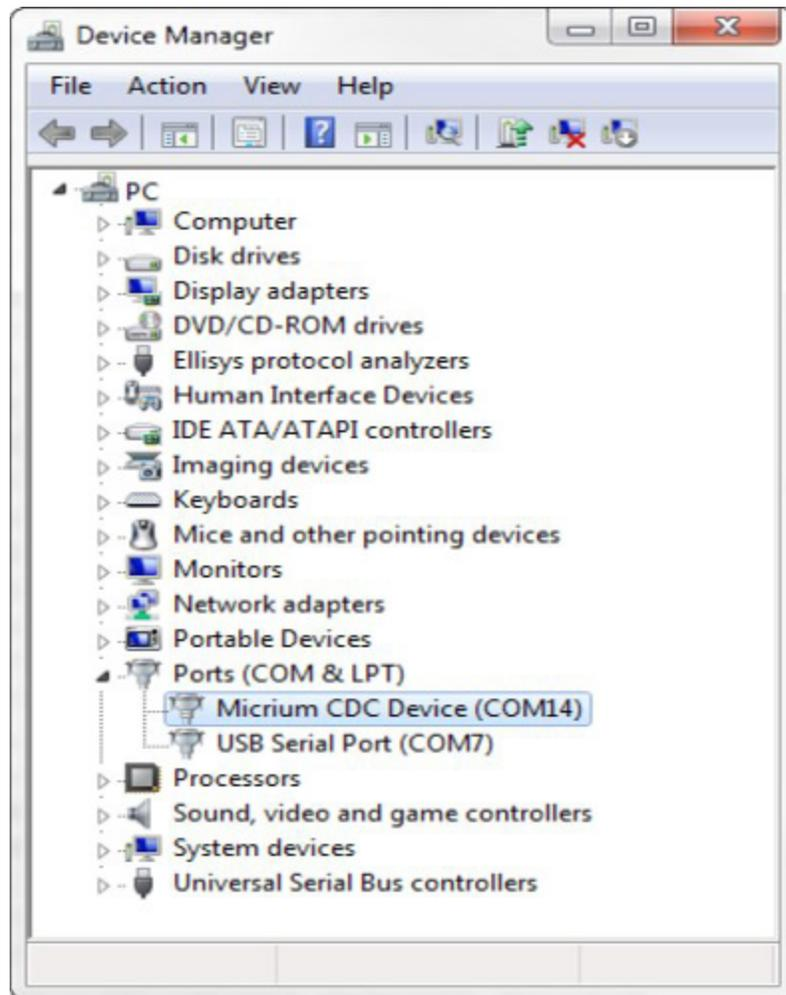
Figure - Windows Device Manager and Created Virtual COM Port
