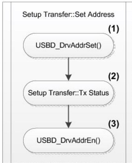
Figure - Device Set Address Diagram
