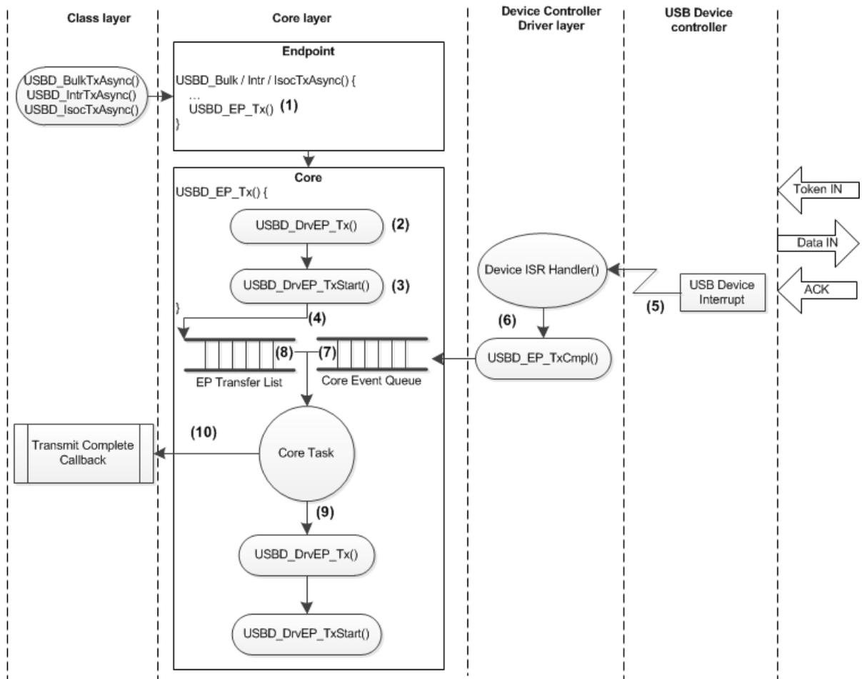
Figure - Device Asynchronous Transmit Diagram
