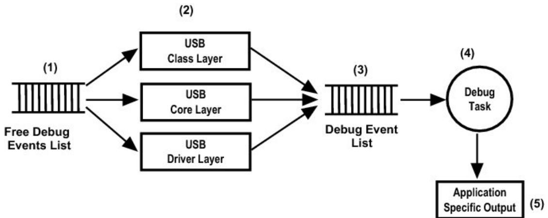
Figure - Processing USB Debug Events
