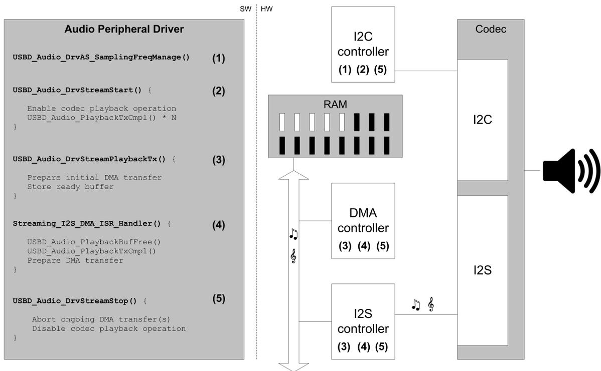
Figure - Playback Stream Functions
