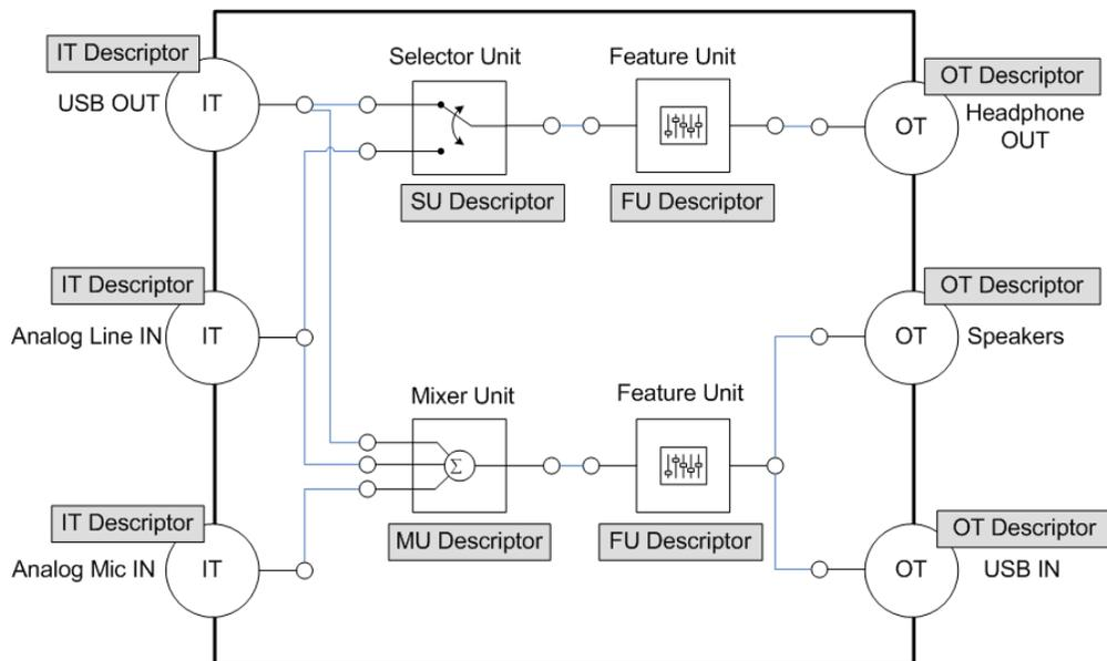
Figure - Example of Audio Function Topology
