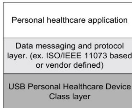
Figure - Personal Healthcare Device Software Layers
