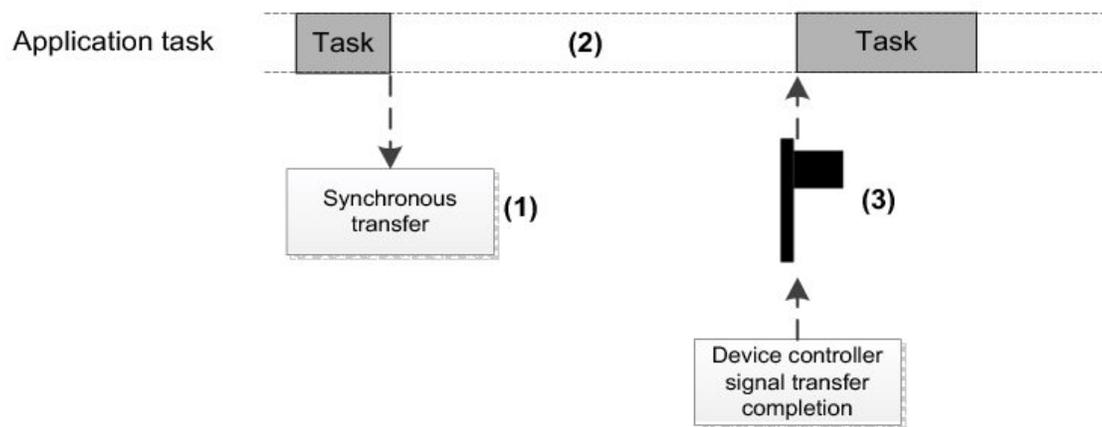
Figure - Synchronous transfer completion notification
