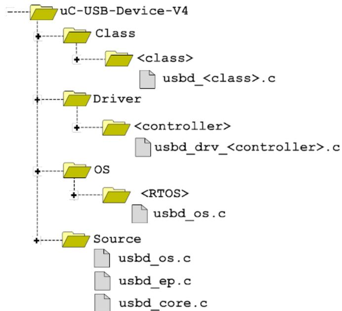
Figure - µC/USB-Device Source Code
