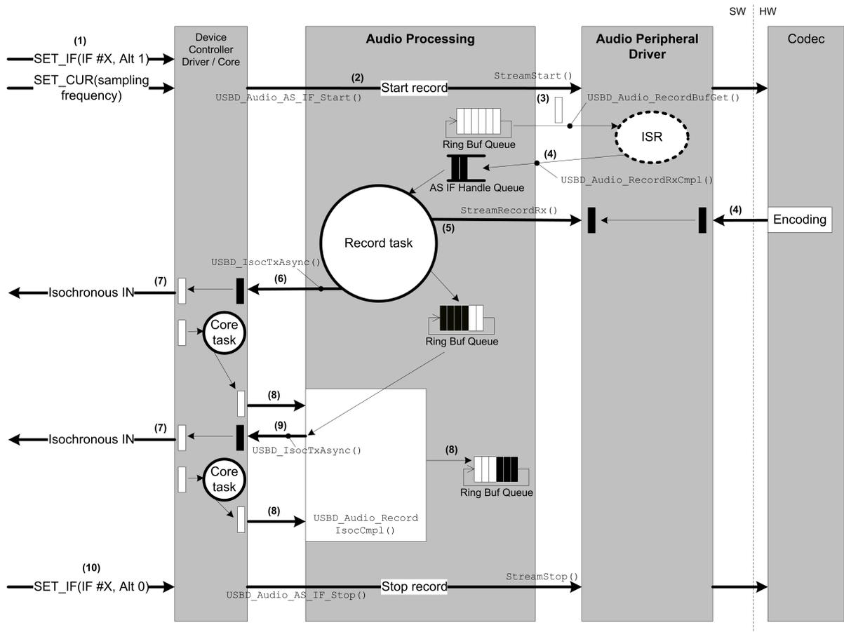
Figure - Record Stream Dataflow
