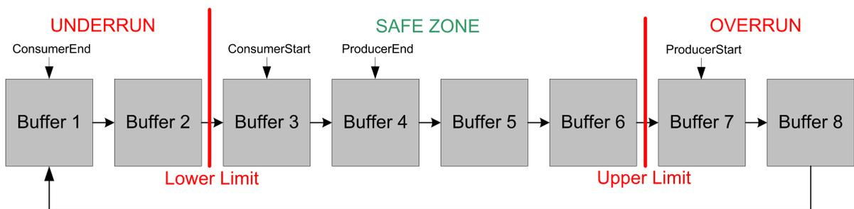
Figure - Playback Ring Buffers Queue Monitoring
