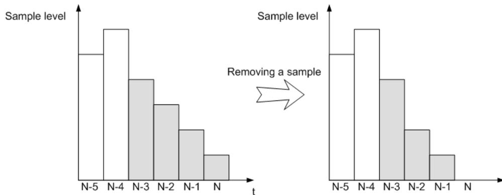
Figure - Removing a Sample in Case of Overrun
