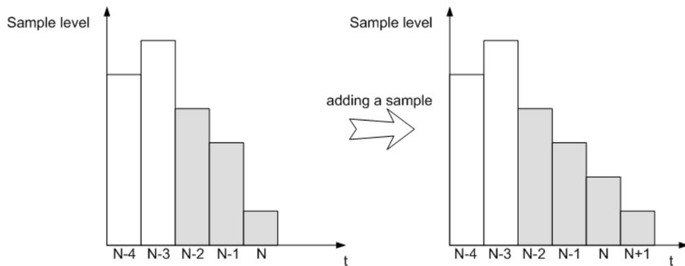
Figure - Adding a Sample in Case of Underrun
