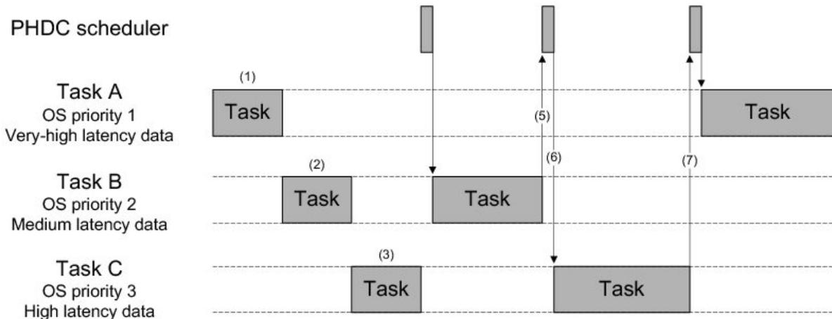
Figure - Task Execution Order, with QoS Based Scheduling
