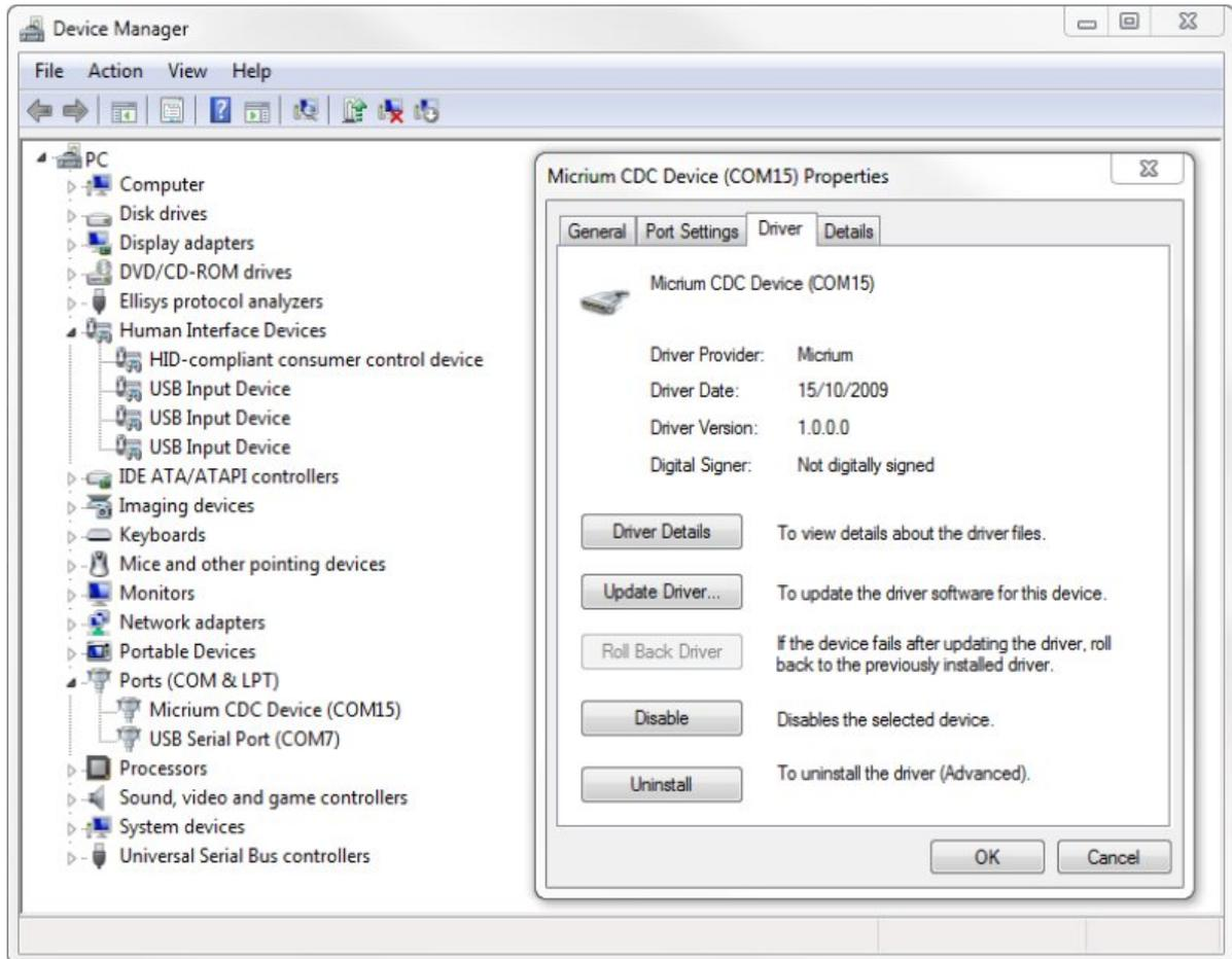
Figure - Windows Device Manager Example for a CDC Device
