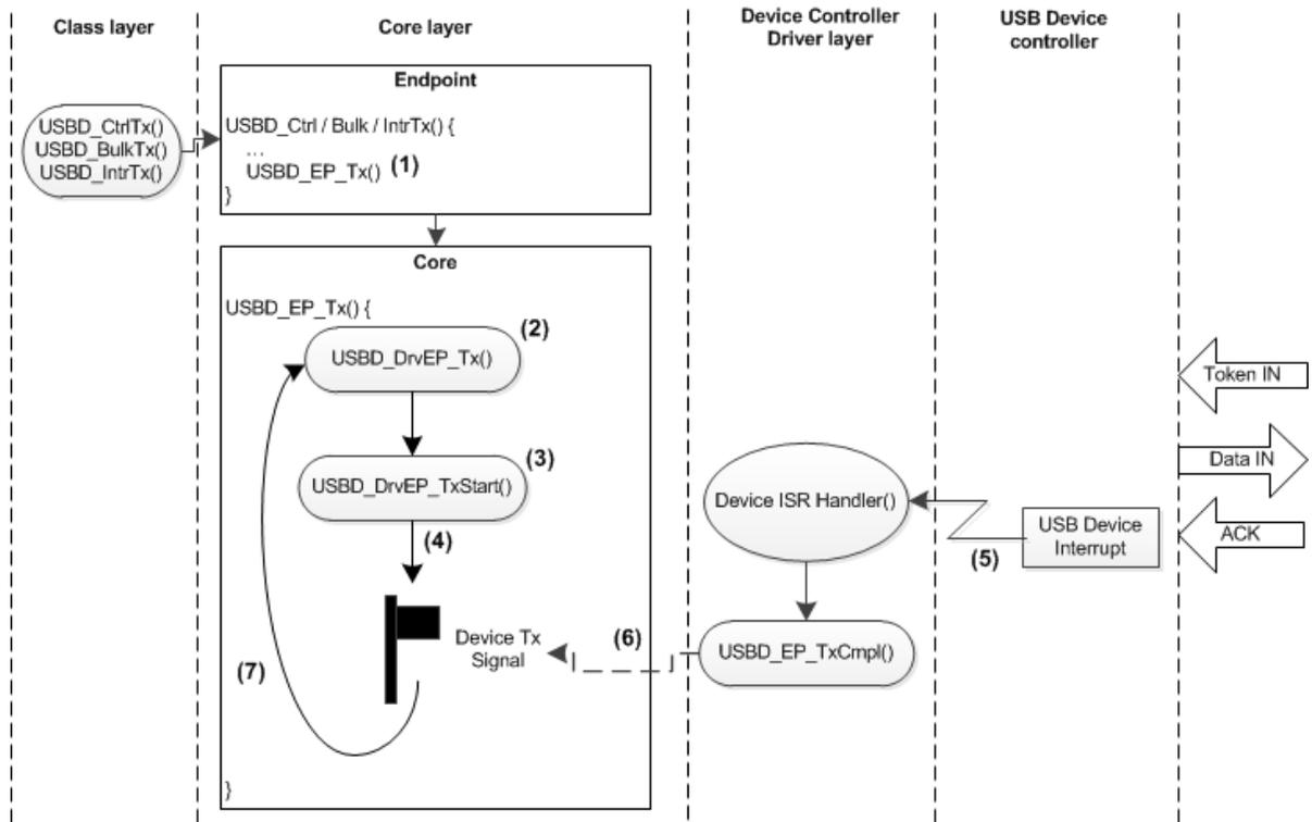
Figure - Device Synchronous Transmit Diagram
