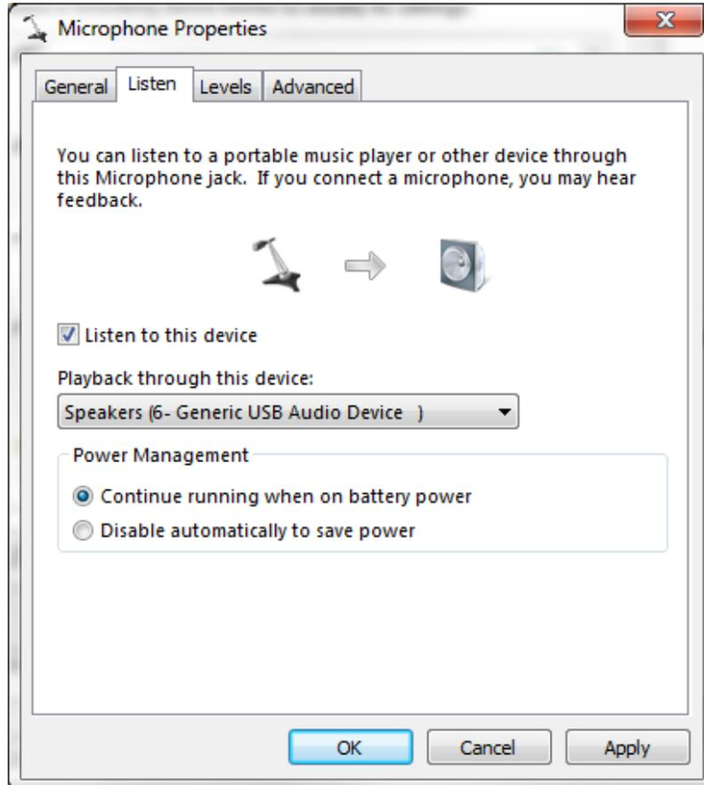
Figure - Sound Manager - Microphone Playthrough for Loopback Demo
