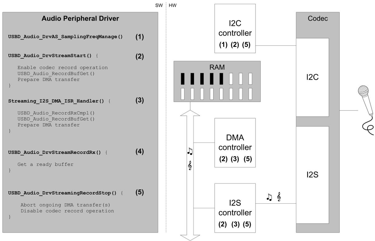
Figure - Record Stream Functions
