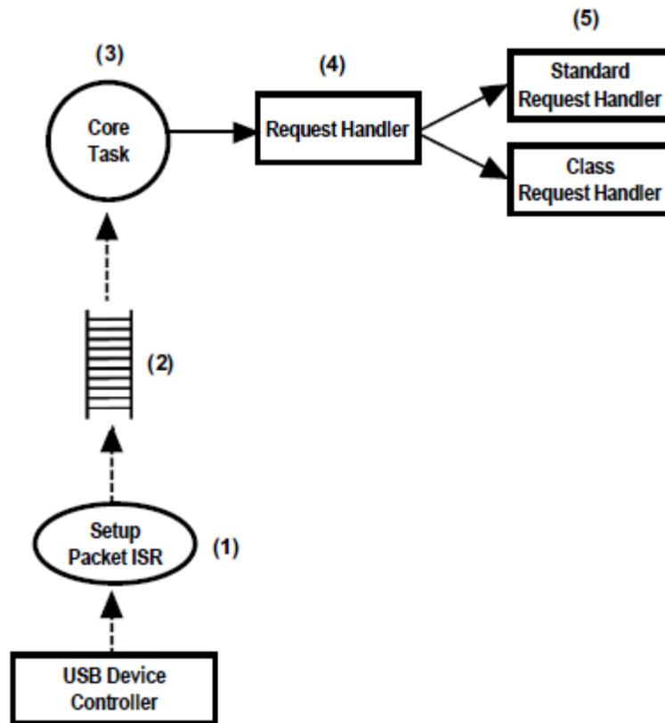
Figure - Processing Setup Packets (USB Requests)
