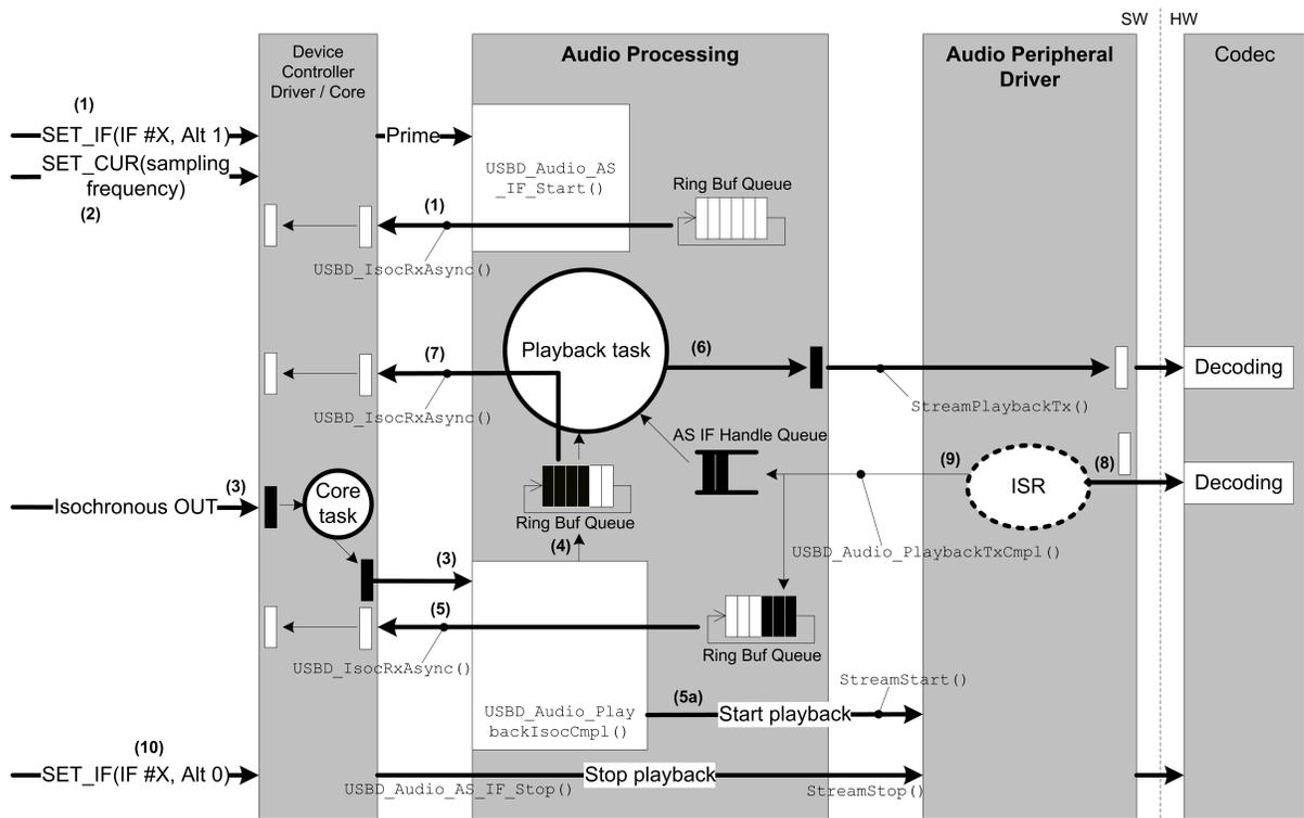
Figure - Playback Stream Dataflow
