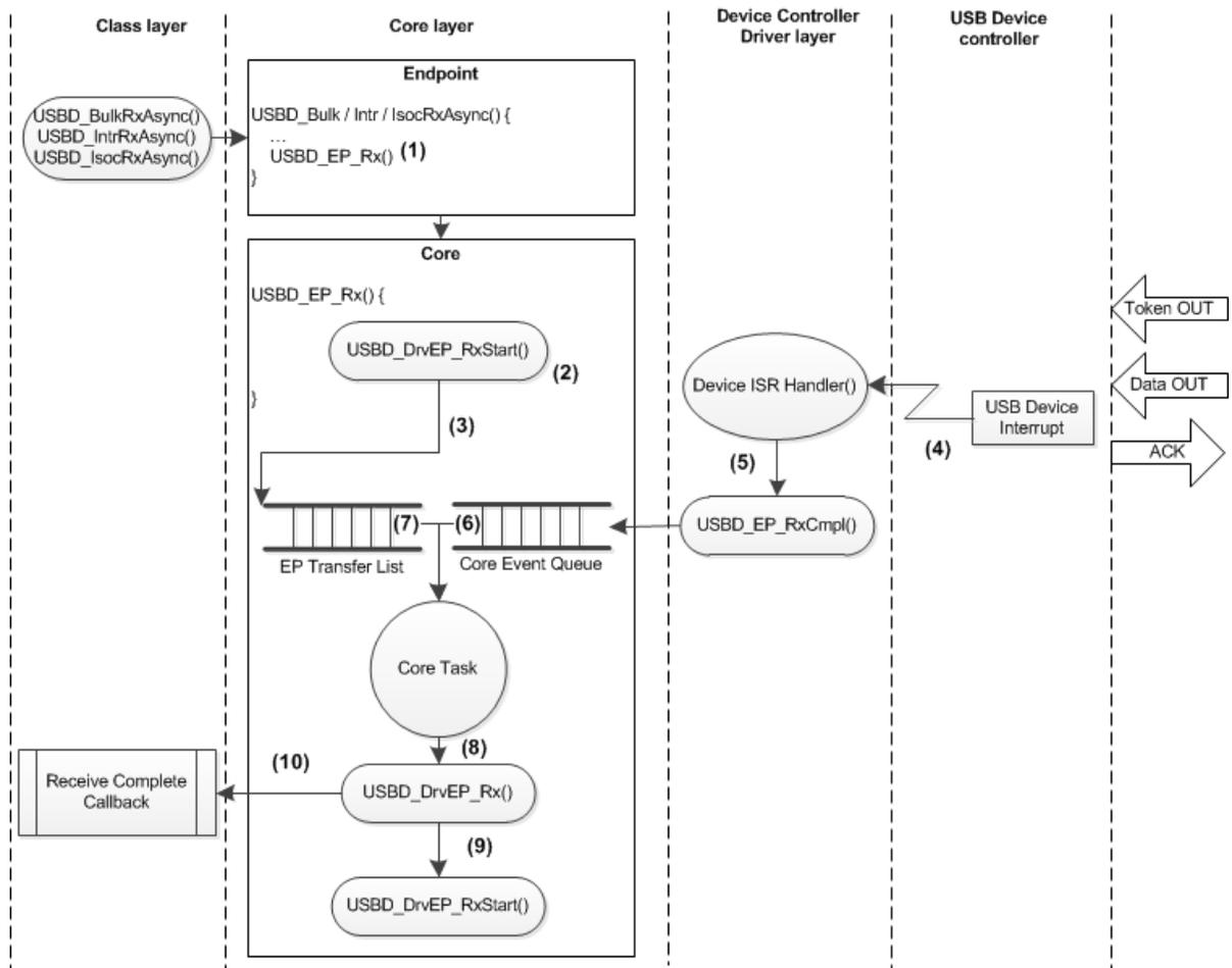
Figure - Device Asynchronous Receive Diagram
