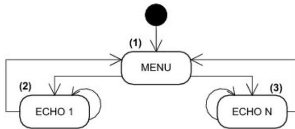
Figure - Serial Demo State Machine
