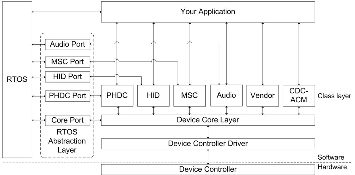
Figure - µC/USB-Device architecture with RTOS interactions
