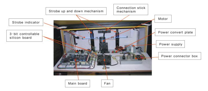
Motor: Drives the strobe mechanism.
