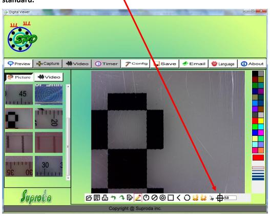
2. Put the Digital Viewer microscope on the Calibration Pattern sheet, you can see the black/white block on the screen.
