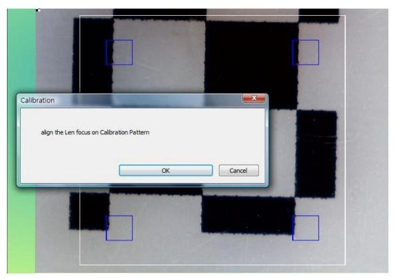
3. Align the Calibration pattern block (black and white) to the white rectangle edge. (To push the "PgUp" key to enlarge the white rectangle or push the "PgDn" to shrink the white rectangle.)
