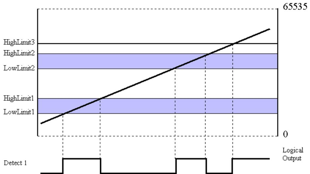
**Example Detection: Channel 1 in Totalizing Counter Mode**
