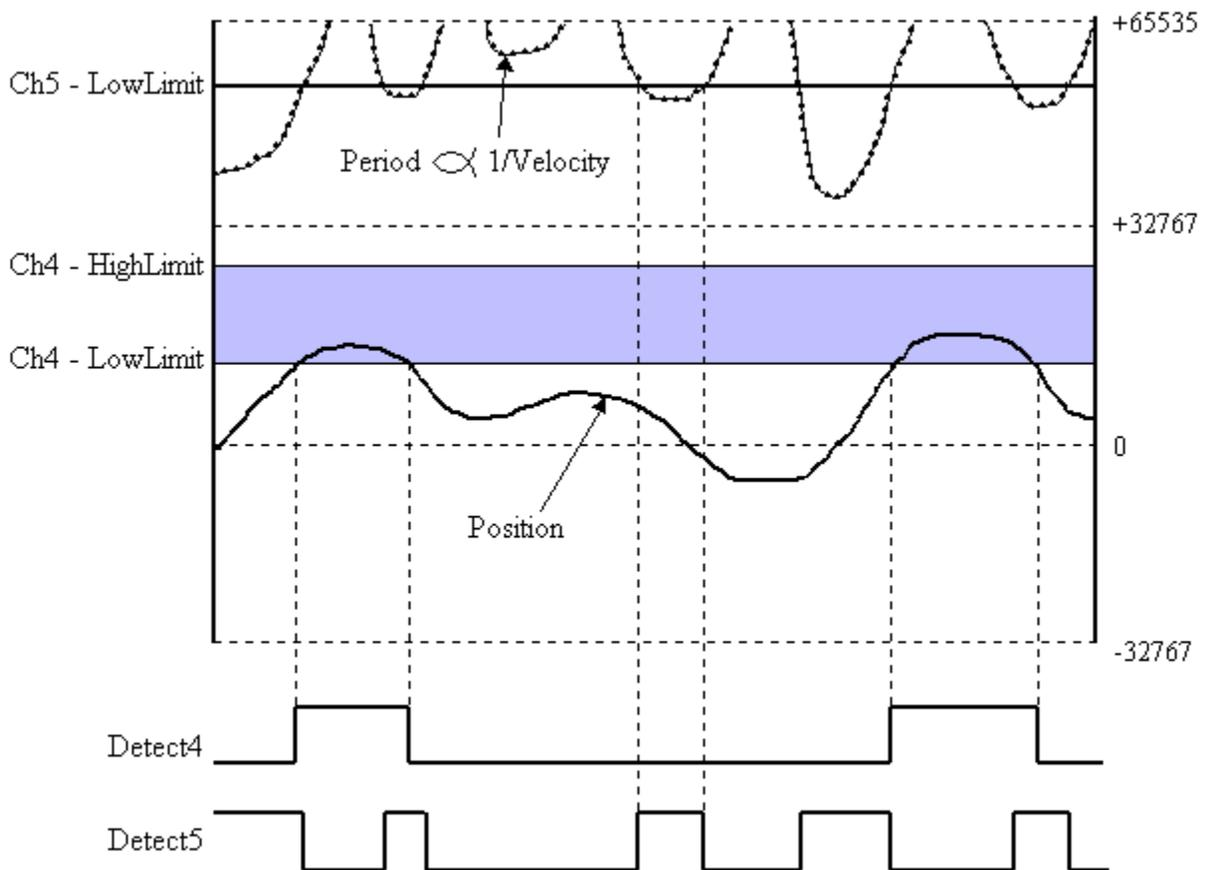
**Detection Example: Channel 4 in Encoder Position Mode, Channel 5 in Period Mode**
