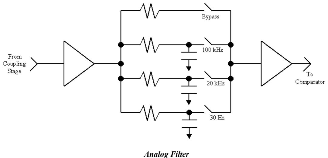
Each channel has a single-pole, low-pass filter with three programmable cut-off frequencies. These are: 100 kHz, 20 kHz, and 30 Hz.
