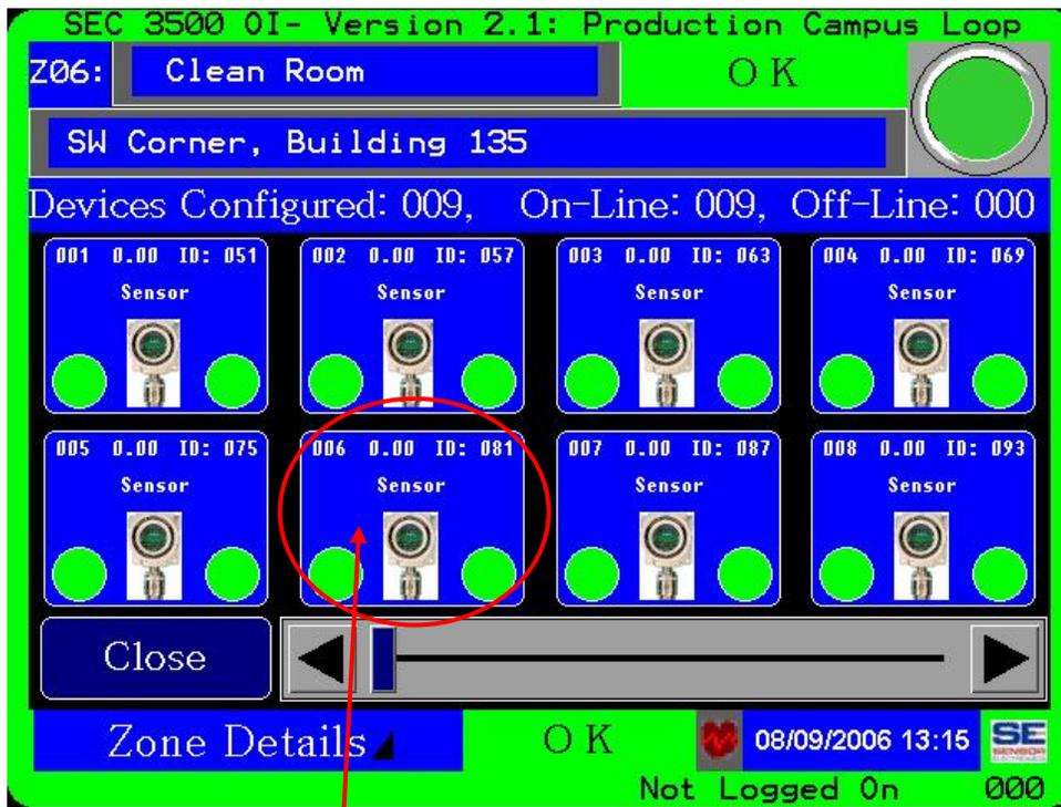
Simply press on the desired device box from the “Zone Details” screen as shown.
