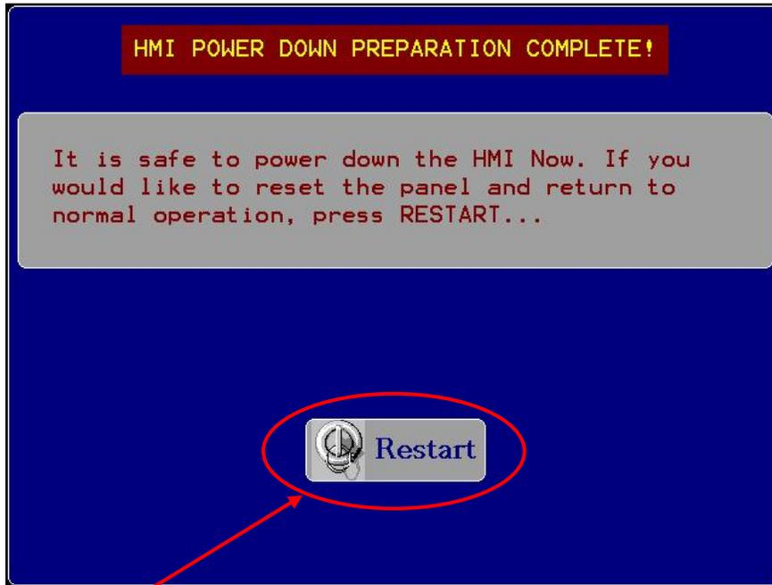
This screen will continue to display every time the panel is powered down until “Restart” above is pressed. So for now, if the intention is to safely shut down; now is the proper time to remove power from the panel. When the panel is power back on, the screen will return. And if you are ready to return to normal operation, then press the “Restart” button, and the following screen will be displayed:
