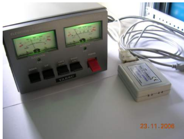
Figure 2.7: WinRotor Computer Interface.
